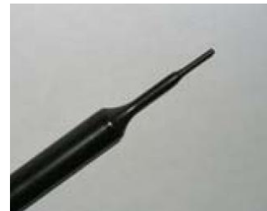
Picture C.2 Near-field Probe
