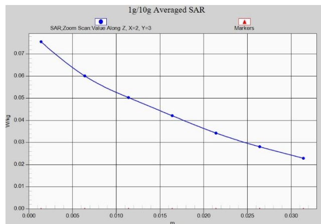
Fig. 1-21 Z-Scan at power reference point (LTE B28 Head)
