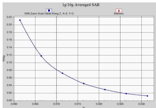
Fig. 1-6 Z-Scan at power reference point (WCDMA850 Body)
