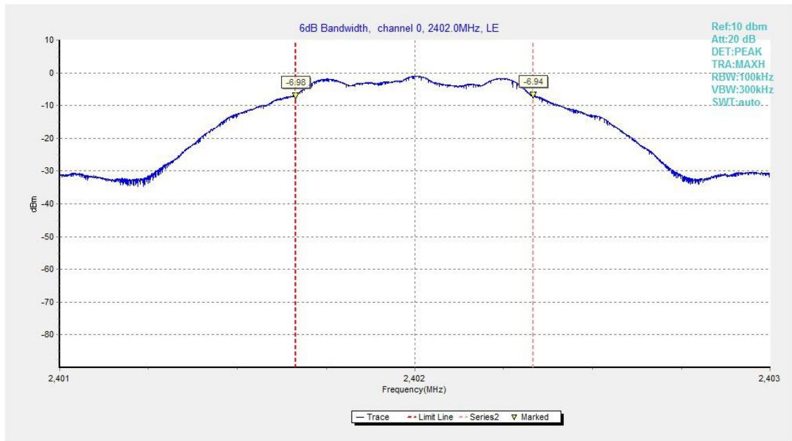
Fig.20. 6dB Bandwidth: GFSK, 2402 MHz
