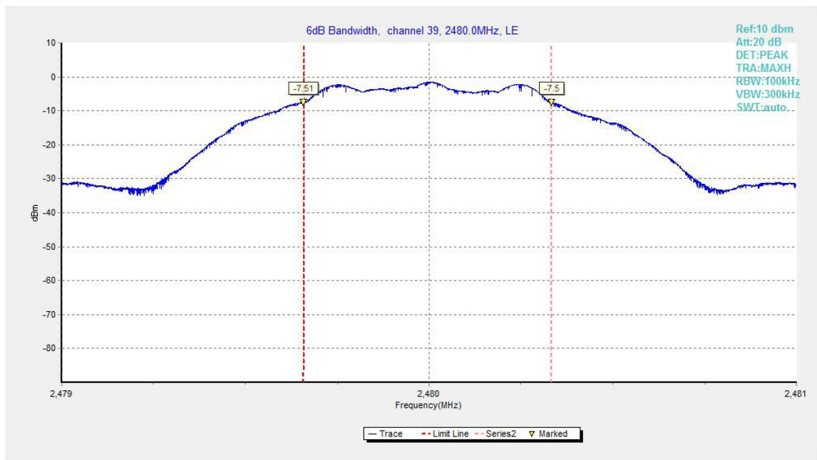
Fig.22. 6dB Bandwidth: GFSK, 2480 MHz
