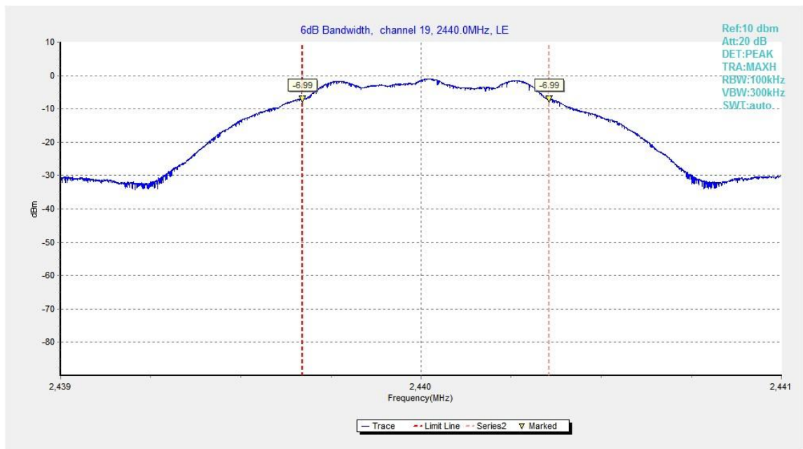
Fig.21. 6dB Bandwidth: GFSK, 2440 MHz
