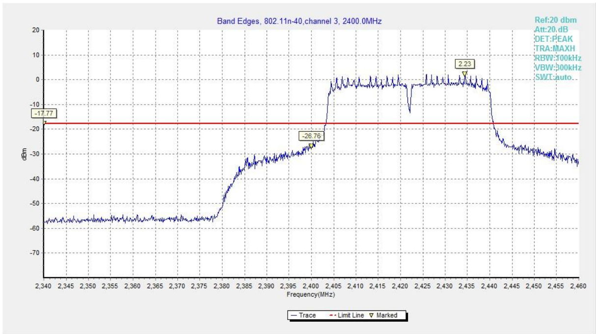
Fig.A.5.7 Band Edges (802.11n-HT40, Ch 3)
