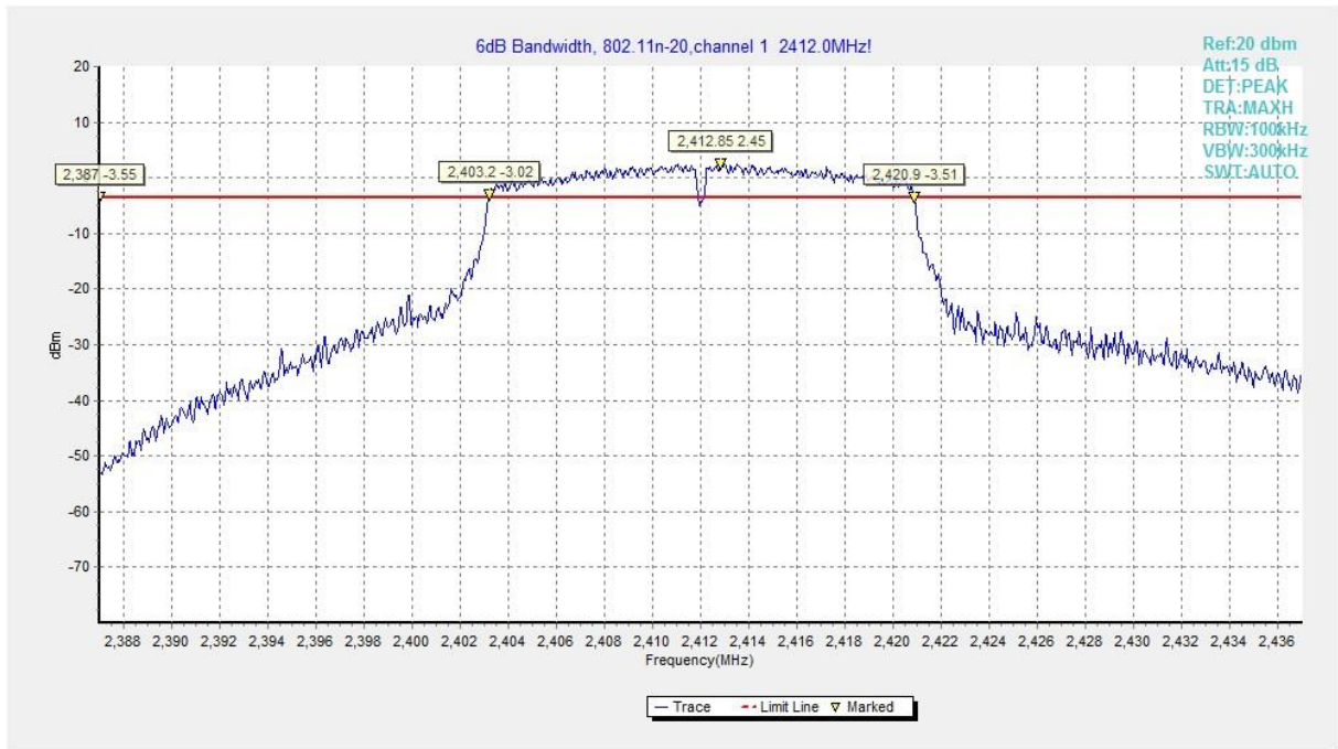
Fig.B.4.7 Occupied 6dB Bandwidth (802.11n-20MHz, Ch 1)
