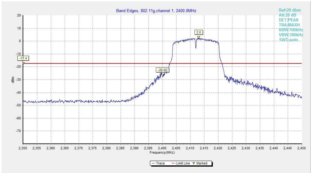
Fig.B.5.3 Band Edges (802.11g, Ch 1)
