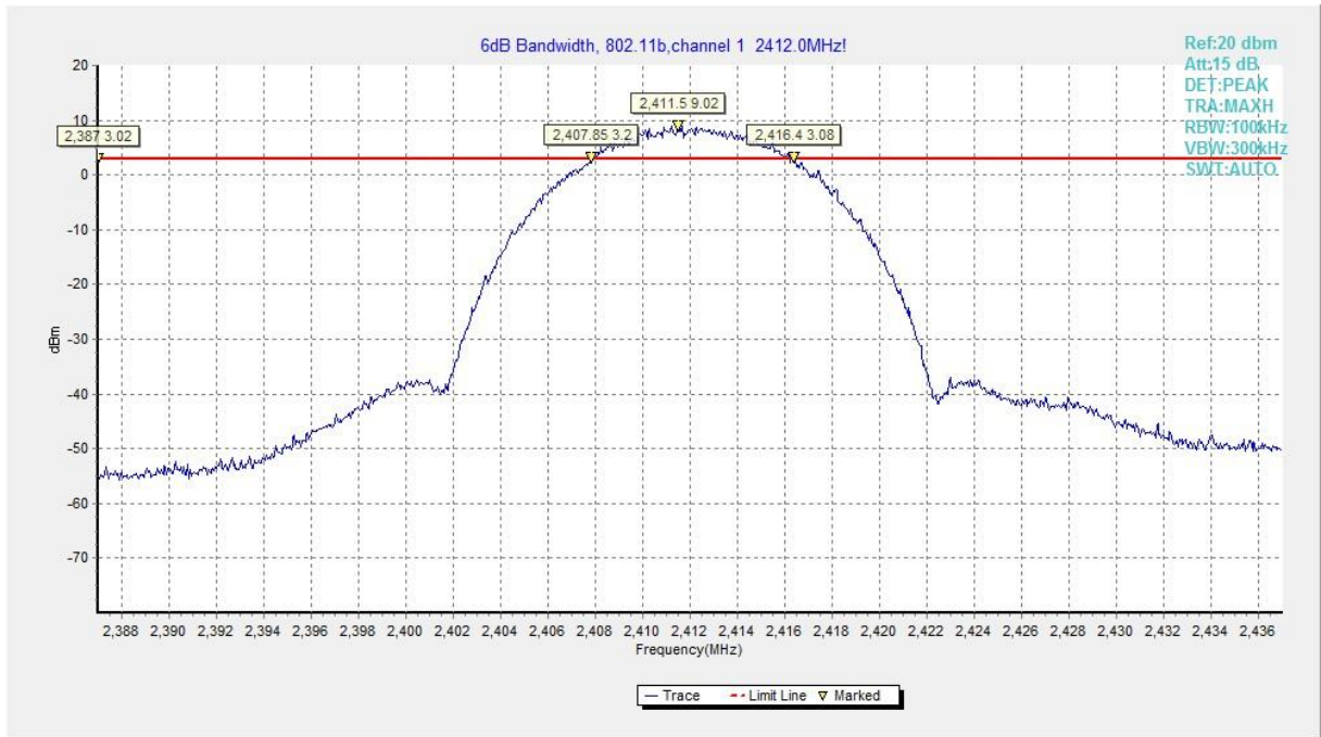
Fig.B.4.1 Occupied 6dB Bandwidth(802.11b,Ch 1)
