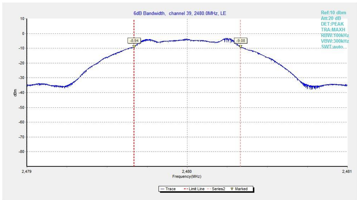
Fig.22. 6dB Bandwidth: GFSK, 2480 MHz
