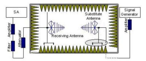
In the chamber, a substitution antenna for the frequency band of interest is placed at the reference point of the chamber. An RF Signal source for the frequency band of interest is connected to the substitution antenna with a cable that has been constructed to not interfere with the radiation pattern of the antenna. A power  $(P_{\text{Mea}})$  is applied to the input of the substitution antenna and adjusts the level of the signal generator output until the value of the
