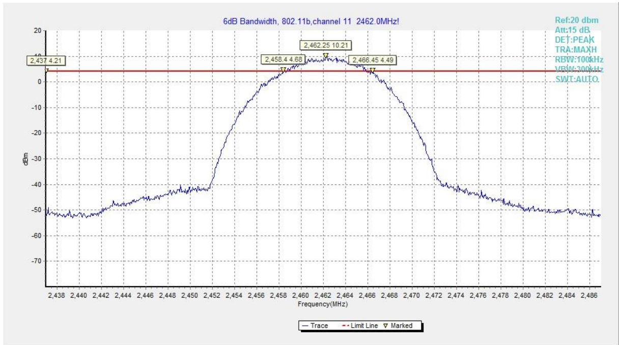
Fig.B.4.3 Occupied 6dB Bandwidth (802.11b, Ch 11)
