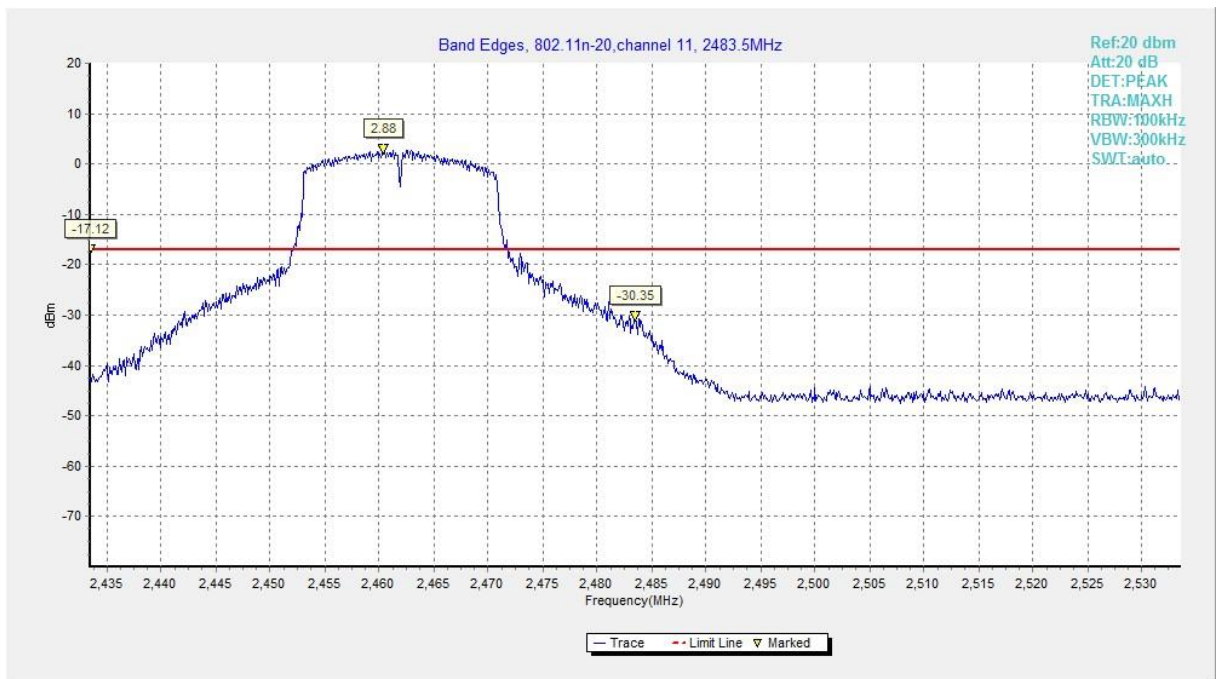
Fig.B.5.6 Band Edges (802.11n-HT20, Ch 11)
