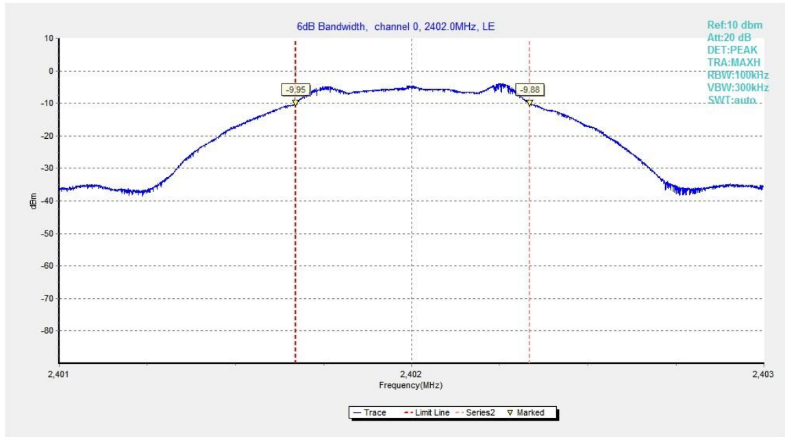
Fig.20. 6dB Bandwidth: GFSK, 2402 MHz
