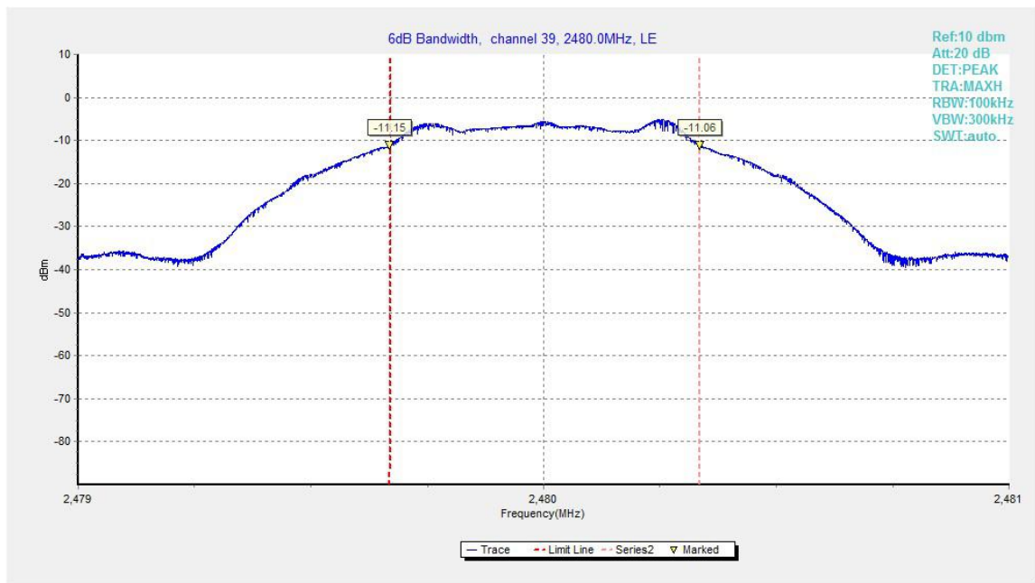
Fig.22. 6dB Bandwidth: GFSK, 2480 MHz
