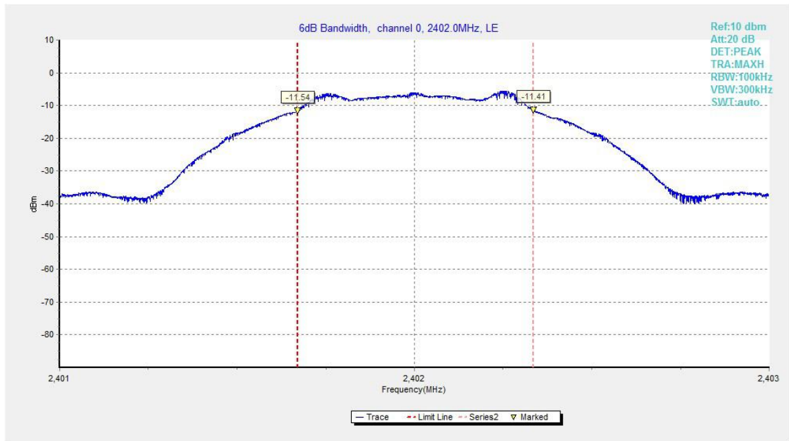
Fig.20. 6dB Bandwidth: GFSK, 2402 MHz
