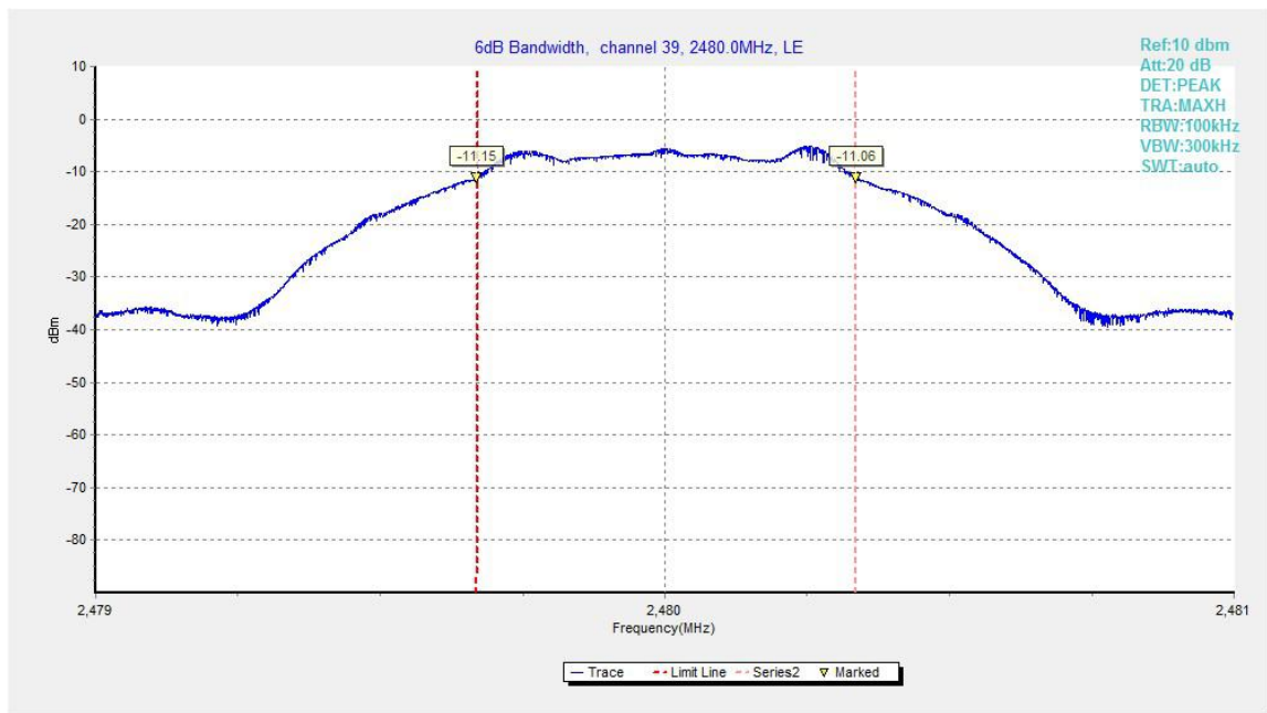
Fig.22. 6dB Bandwidth: GFSK, 2480 MHz
