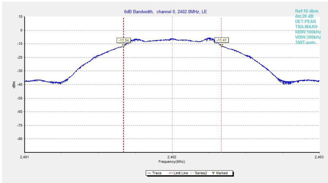
Fig.20. 6dB Bandwidth: GFSK, 2402 MHz
