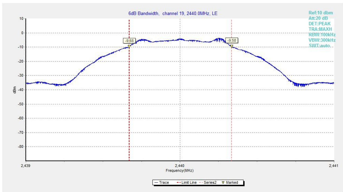
Fig.21. 6dB Bandwidth: GFSK, 2440 MHz
