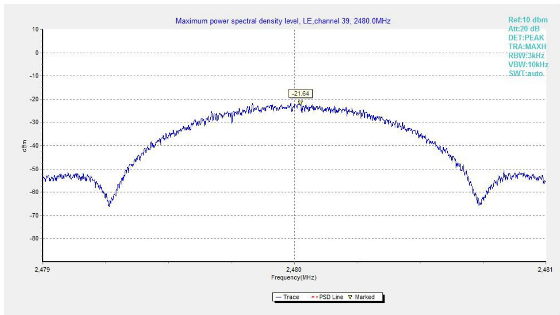
Fig.25. Maximum Power Spectral Density Level Function: GFSK, 2480 MHz
