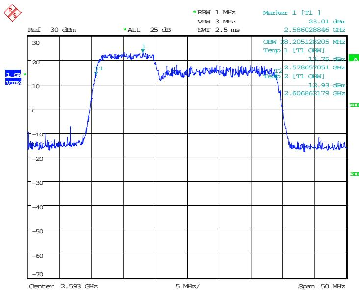
**LTE band 41 HPUE, 10MHz+20MHz Bandwidth,16QAM (99% BW)**
