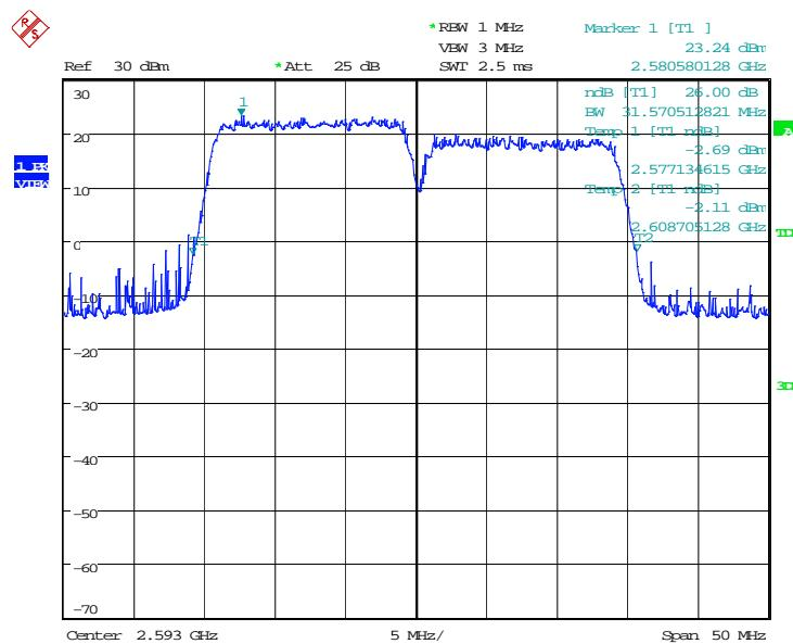
**LTE band 41 HPUE, 15MHz+15MHz Bandwidth,16QAM (-26dBc BW)**
