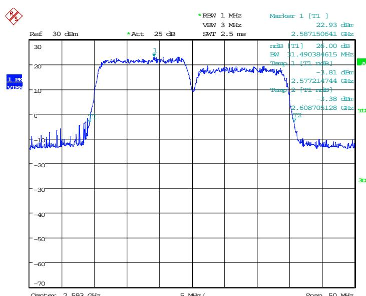
**LTE band 41 HPUE, 15MHz+15MHz Bandwidth,64QAM (-26dBc BW)**
