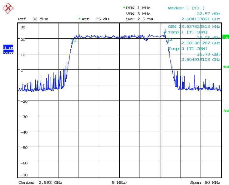
**LTE band 41 HPUE, 20MHz+5MHz Bandwidth,16QAM (99% BW)**
