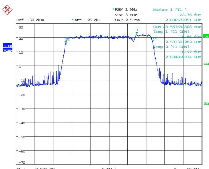
**LTE band 41 HPUE, 20MHz+5MHz Bandwidth,64QAM (99% BW)**
