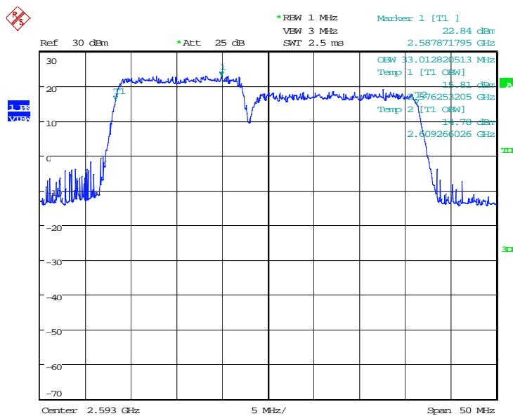
**LTE band 41 HPUE, 15MHz+20MHz Bandwidth,16QAM (99% BW)**
