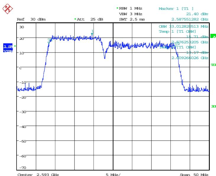
**LTE band 41 HPUE, 15MHz+20MHz Bandwidth,64QAM (99% BW)**
