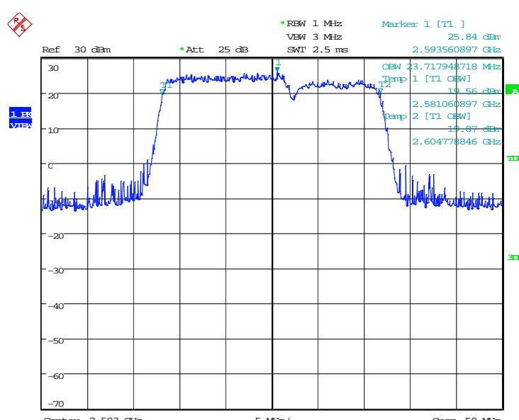
**LTE band 41 HPUE, 15MHz+10MHz Bandwidth,64QAM (99% BW)**
