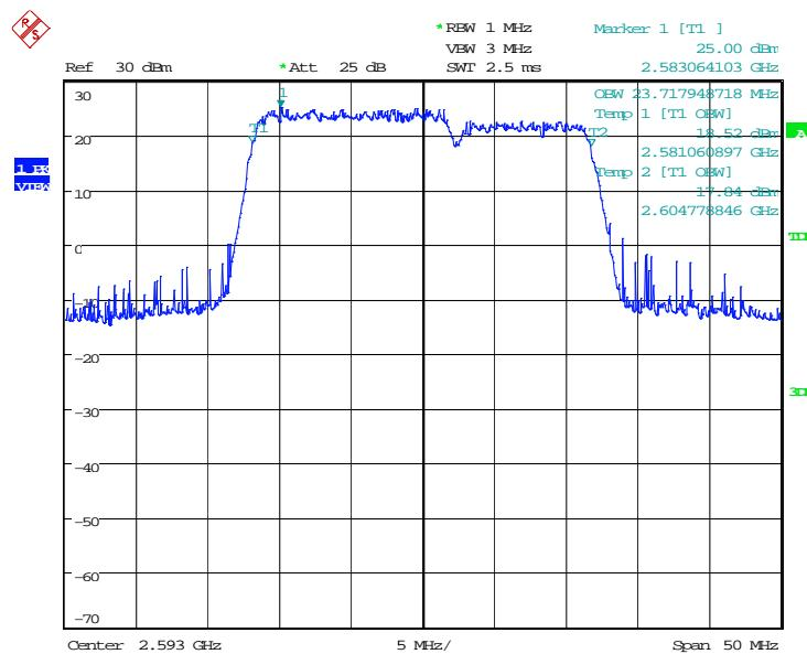
**LTE band 41 HPUE, 15MHz+10MHz Bandwidth,16QAM (99% BW)**
