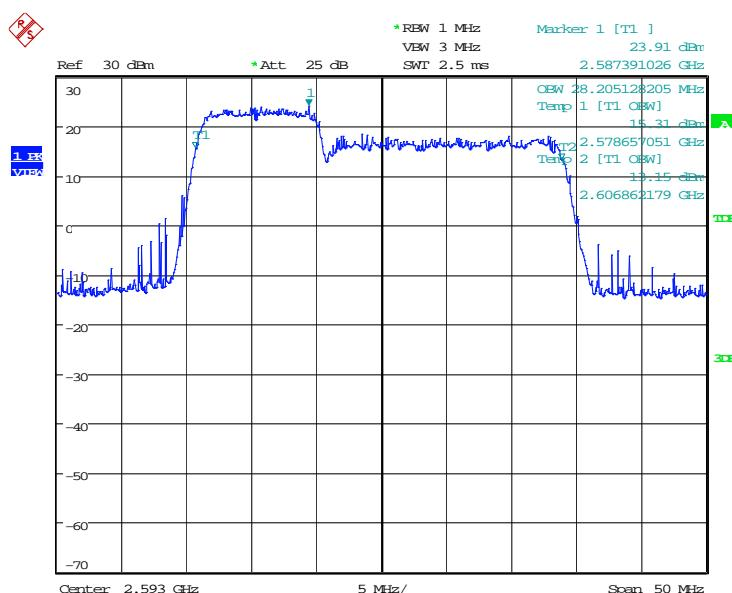
**LTE band 41 HPUE, 10MHz+20MHz Bandwidth,64QAM (99% BW)**
