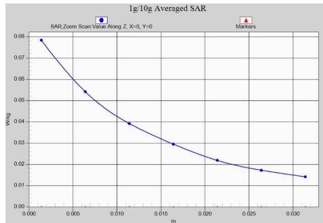
Fig. 13-1 Z-Scan at power reference point (LTE Band2)
