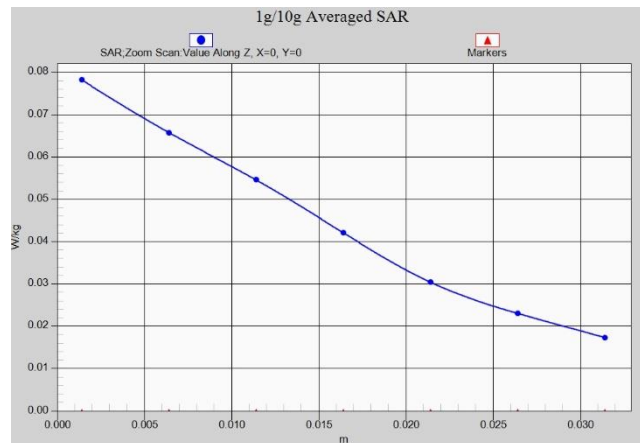
Fig. 4-1 Z-Scan at power reference point (GSM 1900)
