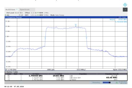
n66,45MHz Bandwidth,DFT-s-QPSK (-26dBc BW)
