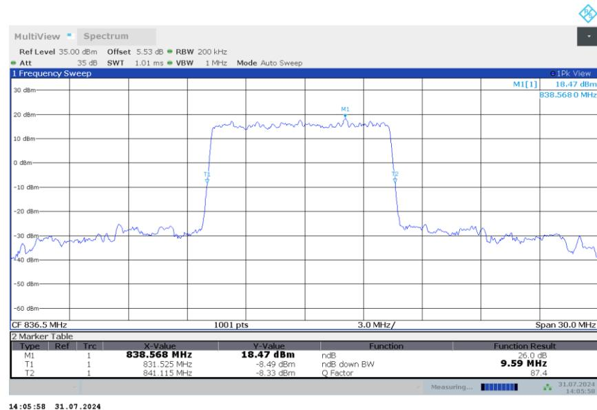
**n5,10MHz Bandwidth,DFT-s-QPSK (-26dBc BW)**
