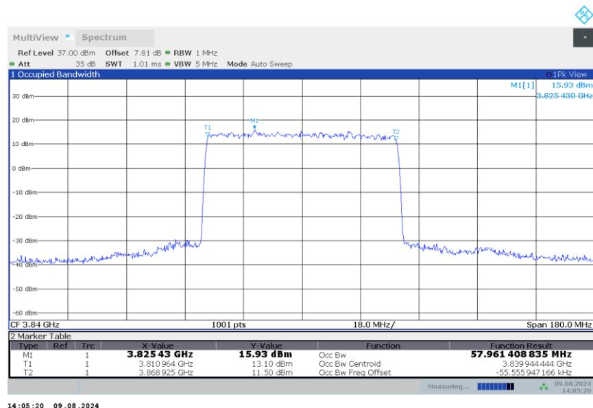
**n77H,60MHz Bandwidth,DFT-s-QPSK (99% BW)**
