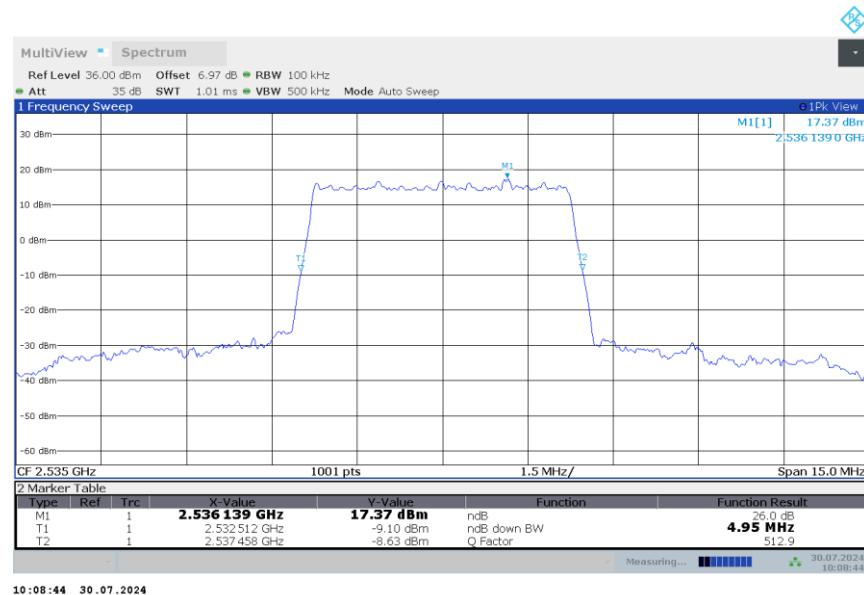
**n7,5MHz Bandwidth,DFT-s-QPSK (-26dBc BW)**
