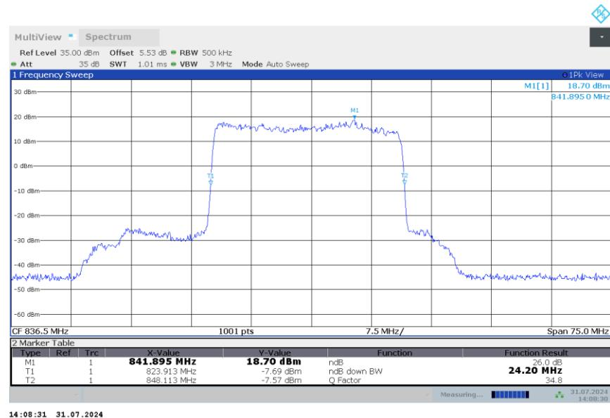
**n5,25MHz Bandwidth,DFT-s-QPSK (-26dBc BW)**
