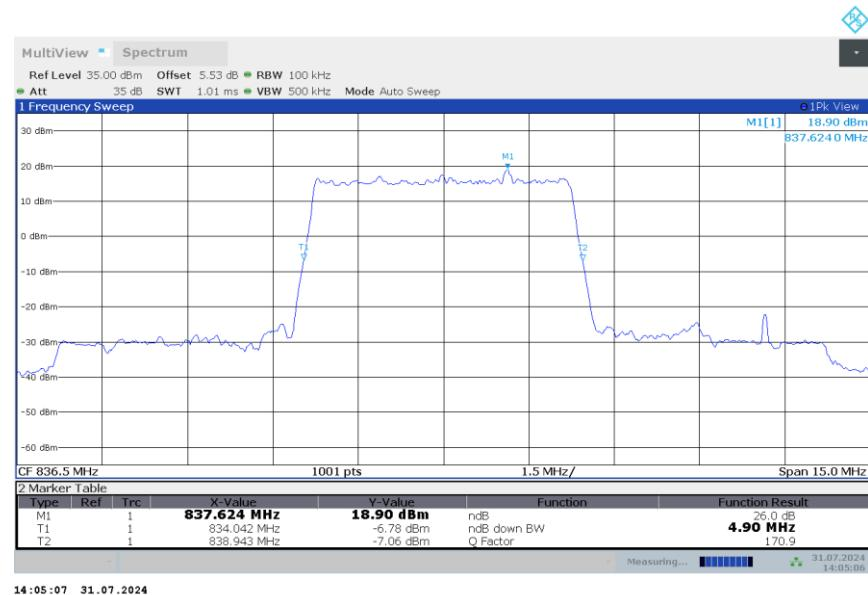
**n5,5MHz Bandwidth,DFT-s-QPSK (-26dBc BW)**
