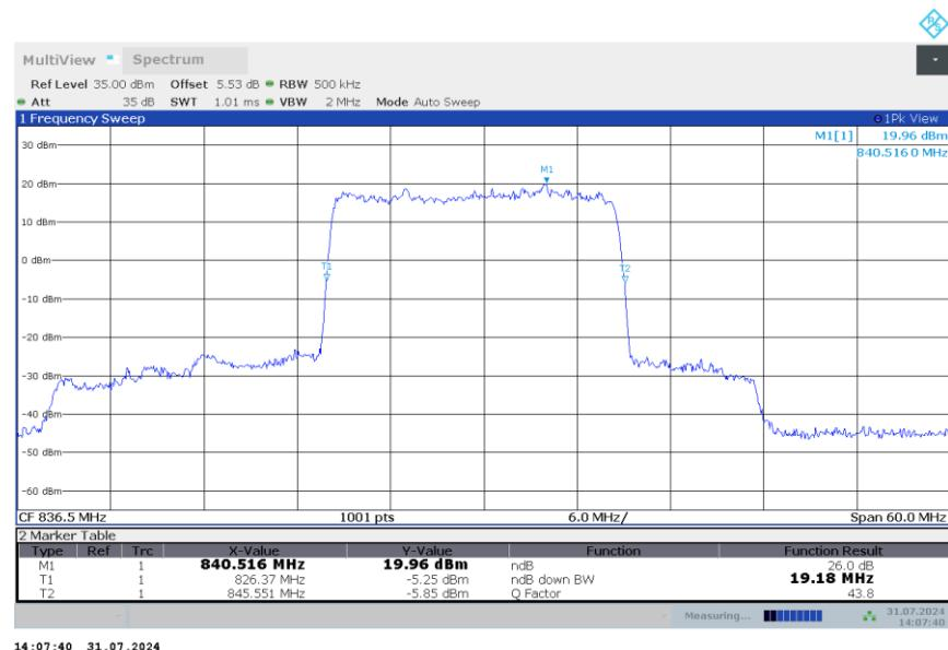
**n5,20MHz Bandwidth,DFT-s-QPSK (-26dBc BW)**
