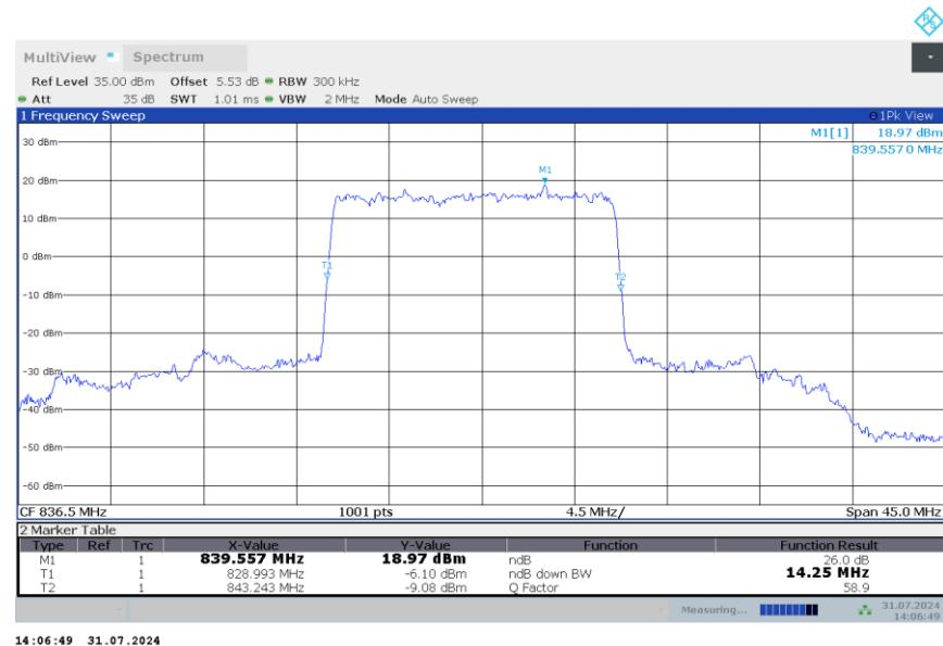
**n5,15MHz Bandwidth,DFT-s-QPSK (-26dBc BW)**
