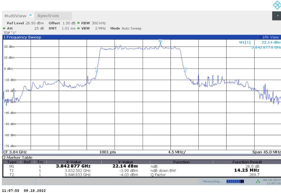
**n77H,15MHz Bandwidth,DFT-s-QPSK (-26dBc BW)**
