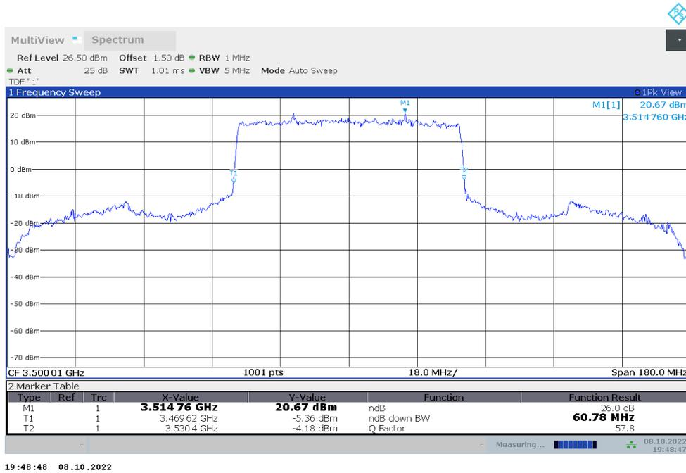
**n77L,60MHz Bandwidth,DFT-s-QPSK (-26dBc BW)**
