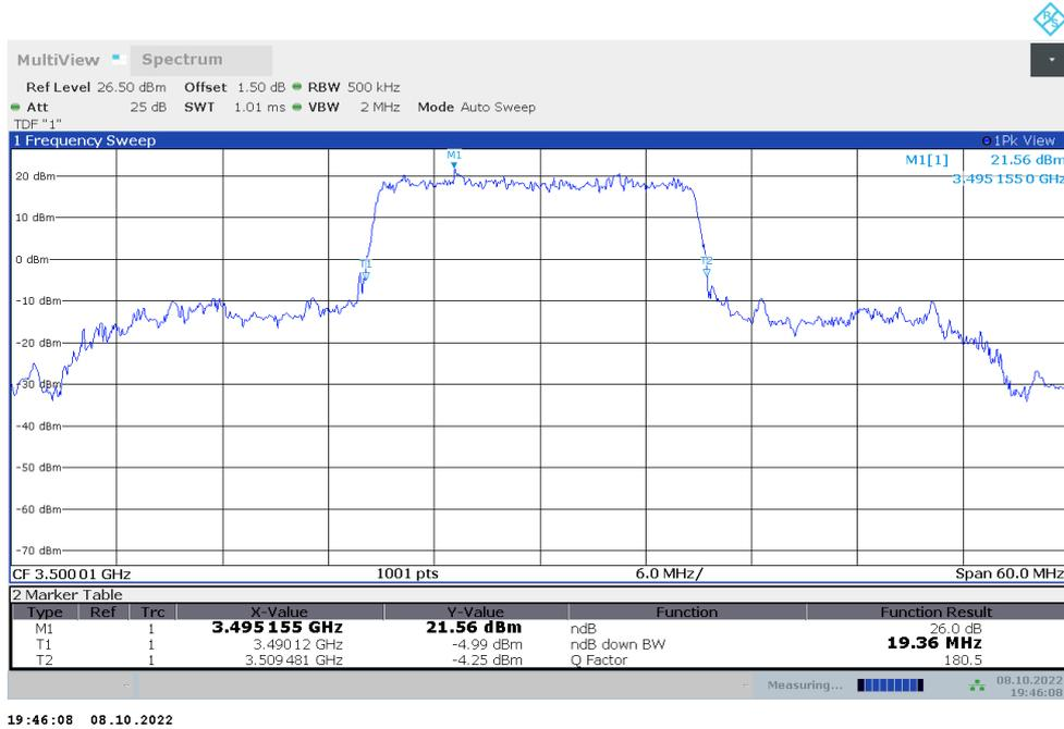
**n77L,20MHz Bandwidth,DFT-s-QPSK (-26dBc BW)**
