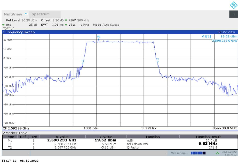
n41,10MHz Bandwidth,DFT-s-QPSK (-26dBc BW)
