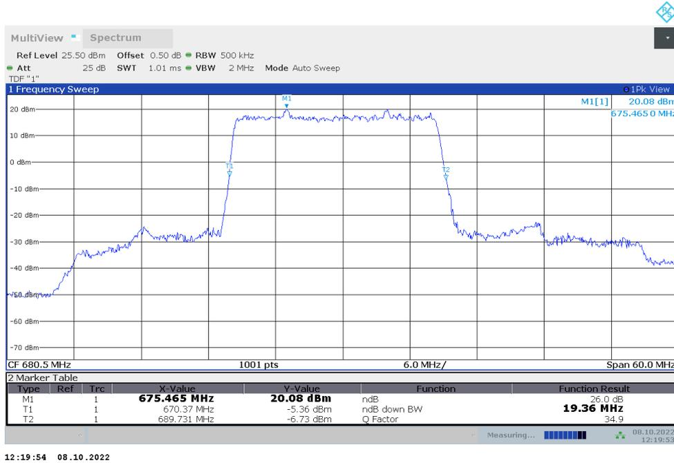
**n71,20MHz Bandwidth,DFT-s-QPSK (-26dBc BW)**
