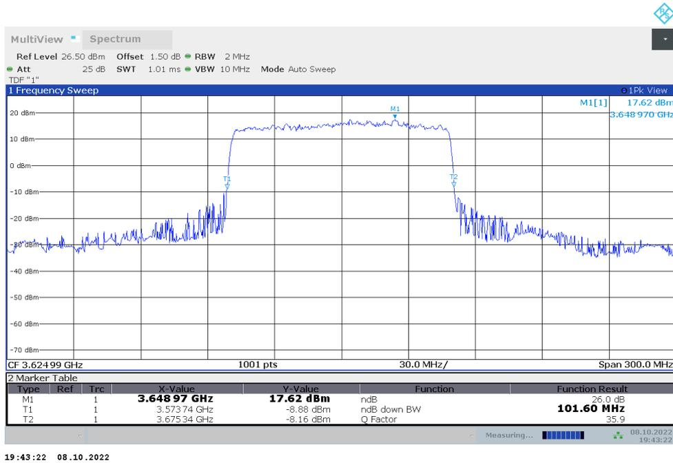
**n48,100MHz Bandwidth,DFT-s-QPSK (-26dBc BW)**
