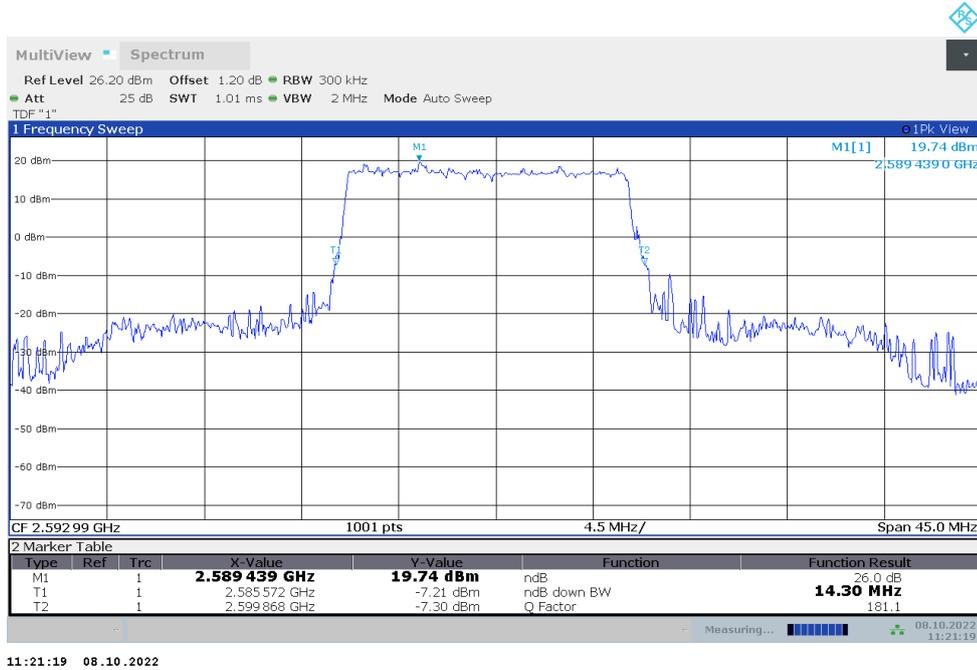
**n41,15MHz Bandwidth,DFT-s-QPSK (-26dBc BW)**
