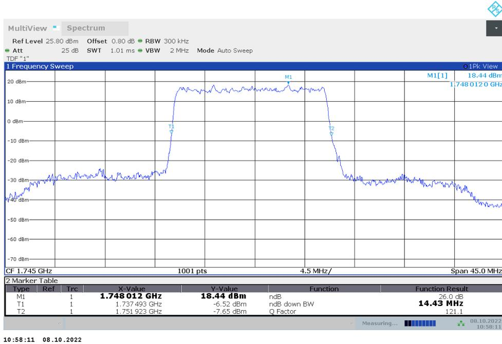
**n66,15MHz Bandwidth,DFT-s-QPSK (-26dBc BW)**
