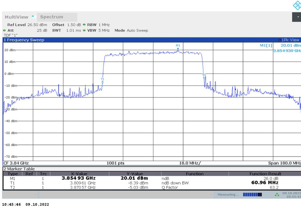
**n77H,60MHz Bandwidth,DFT-s-QPSK (-26dBc BW)**
