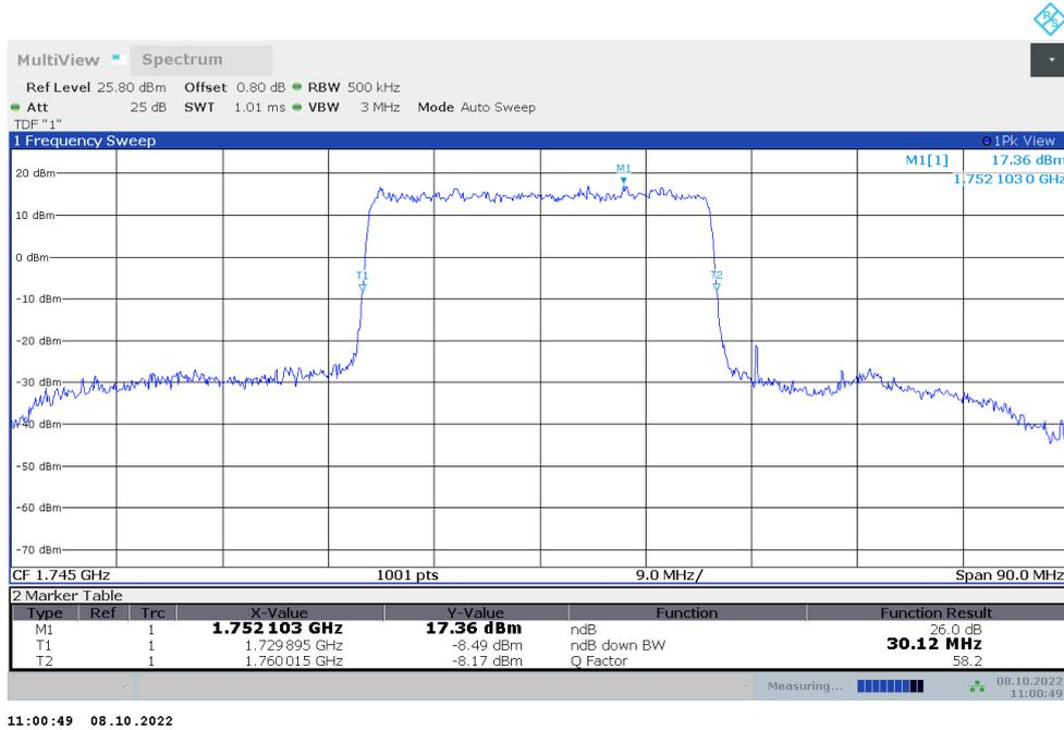
**n66,30MHz Bandwidth,DFT-s-QPSK (-26dBc BW)**
