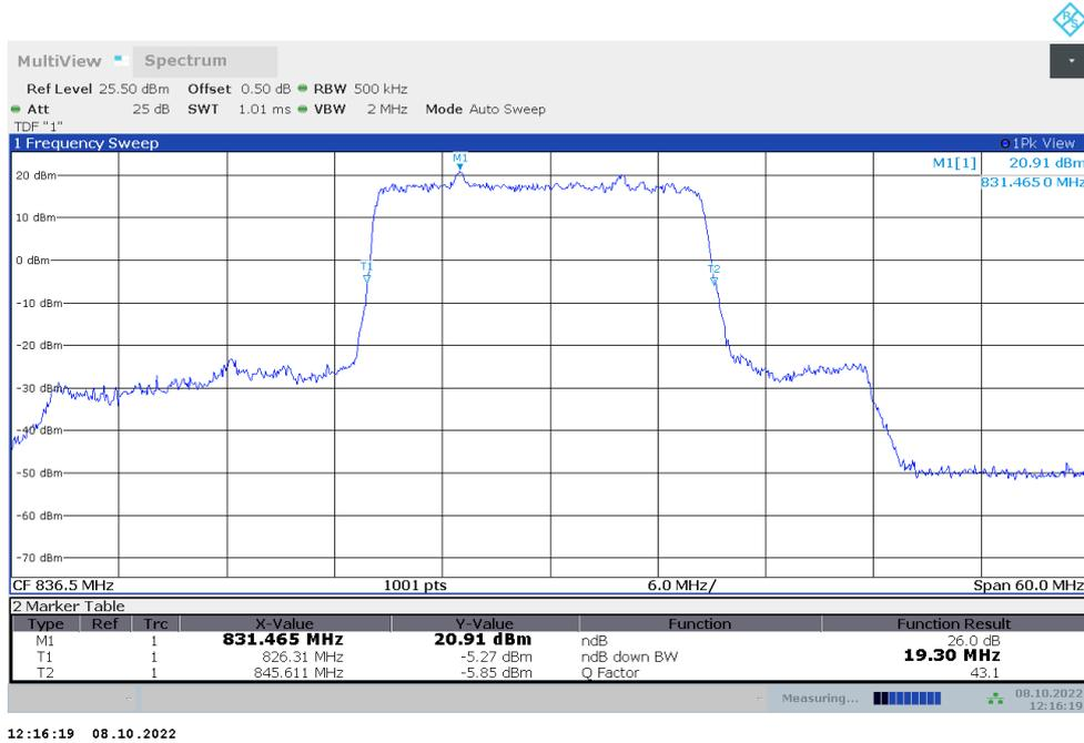
**n5,20MHz Bandwidth,DFT-s-QPSK (-26dBc BW)**
