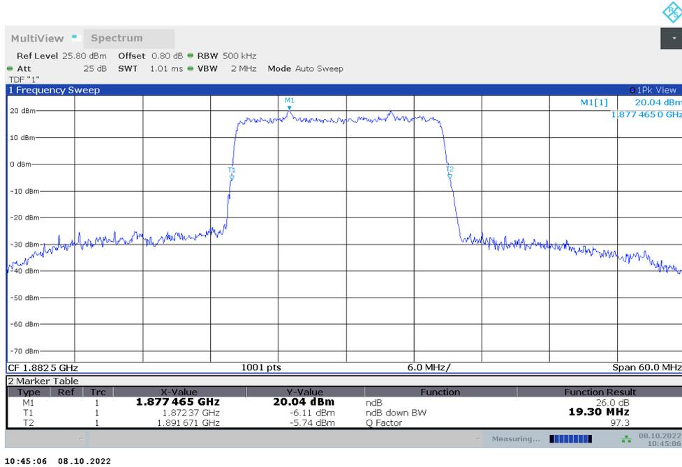
**n25,20MHz Bandwidth,DFT-s-QPSK (-26dBc BW)**
