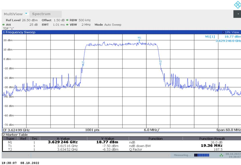
**n48,20MHz Bandwidth,DFT-s-QPSK (-26dBc BW)**
