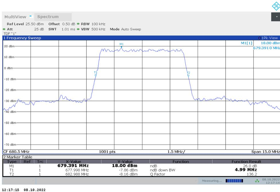
n71,5MHz Bandwidth,DFT-s-QPSK (-26dBc BW)
