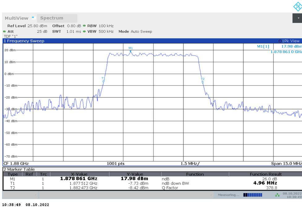
n2,5MHz Bandwidth,DFT-s-QPSK (-26dBc BW)
