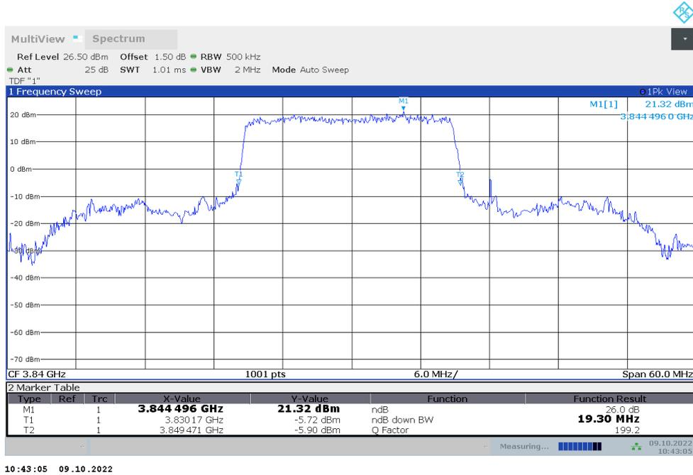
**n77H,20MHz Bandwidth,DFT-s-QPSK (-26dBc BW)**
