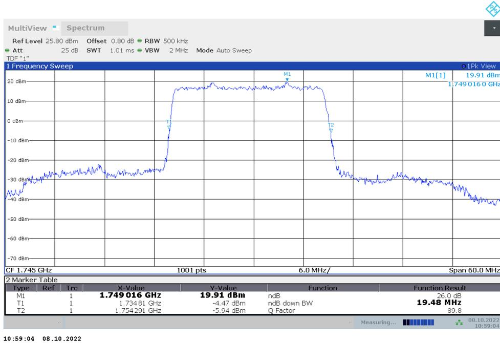
**n66,20MHz Bandwidth,DFT-s-QPSK (-26dBc BW)**
