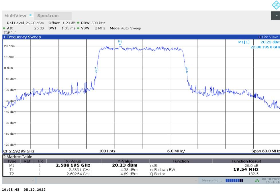
**n41,20MHz Bandwidth,DFT-s-QPSK (-26dBc BW)**
