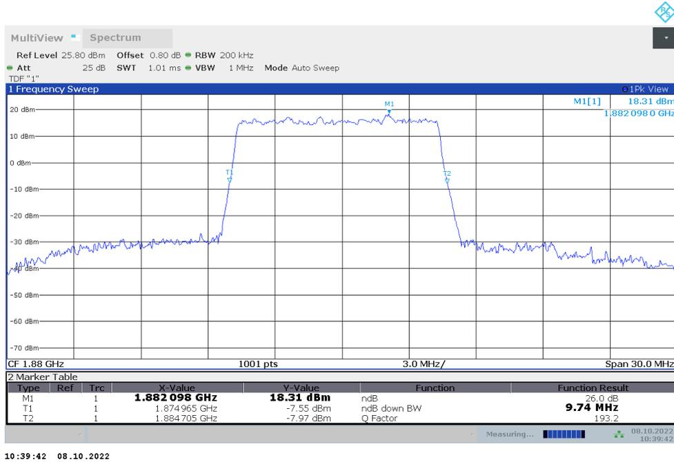
**n2,10MHz Bandwidth,DFT-s-QPSK (-26dBc BW)**
