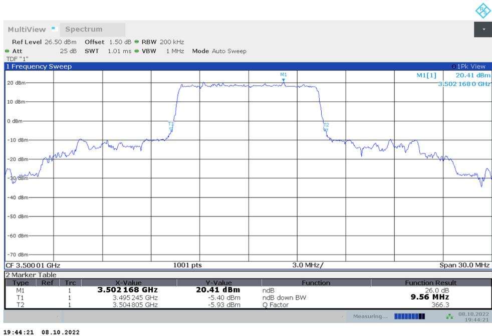
n77L,10MHz Bandwidth,DFT-s-QPSK (-26dBc BW)
