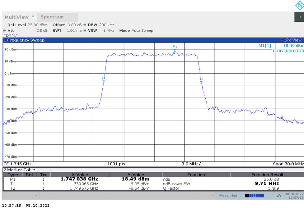
**n66,10MHz Bandwidth,DFT-s-QPSK (-26dBc BW)**
