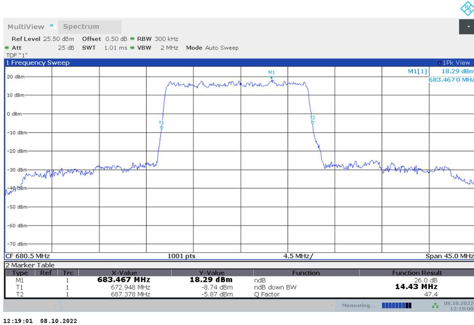
**n71,15MHz Bandwidth,DFT-s-QPSK (-26dBc BW)**
