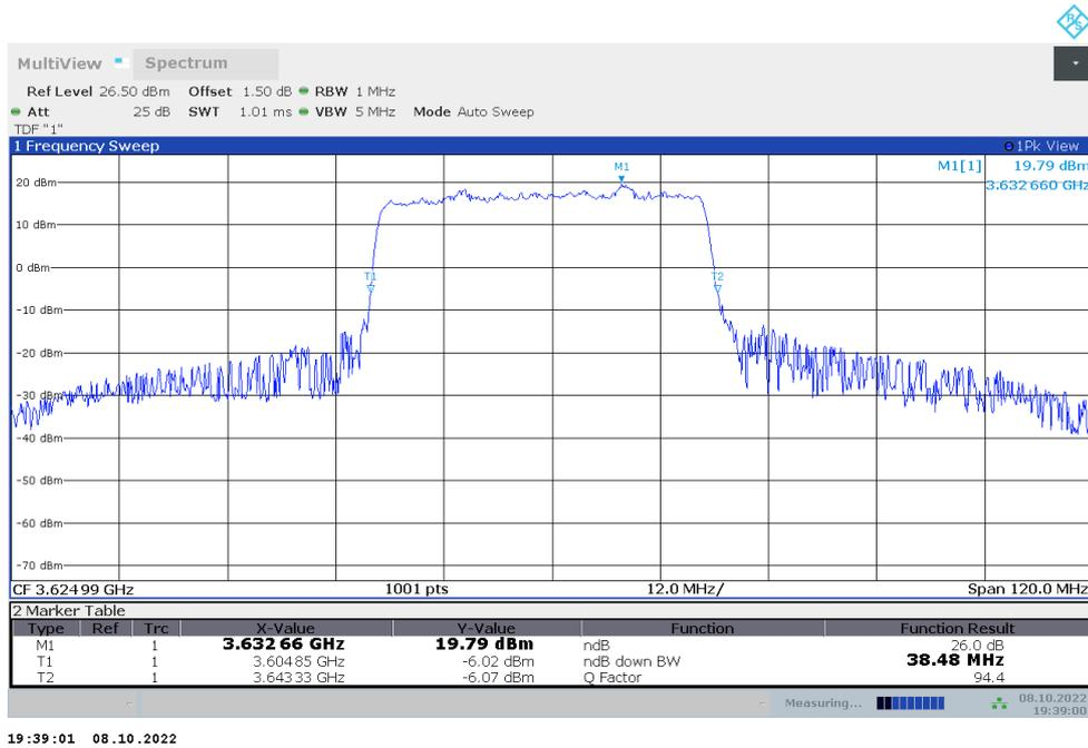
**n48,40MHz Bandwidth,DFT-s-QPSK (-26dBc BW)**
