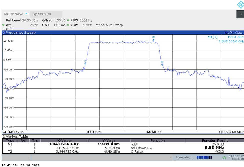
n77H,10MHz Bandwidth,DFT-s-QPSK (-26dBc BW)
