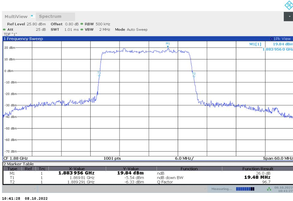
**n2,20MHz Bandwidth,DFT-s-QPSK (-26dBc BW)**
