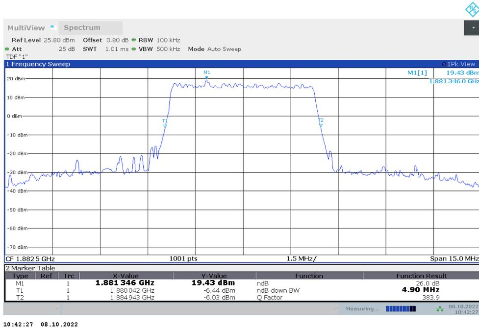
n25,5MHz Bandwidth,DFT-s-QPSK (-26dBc BW)
