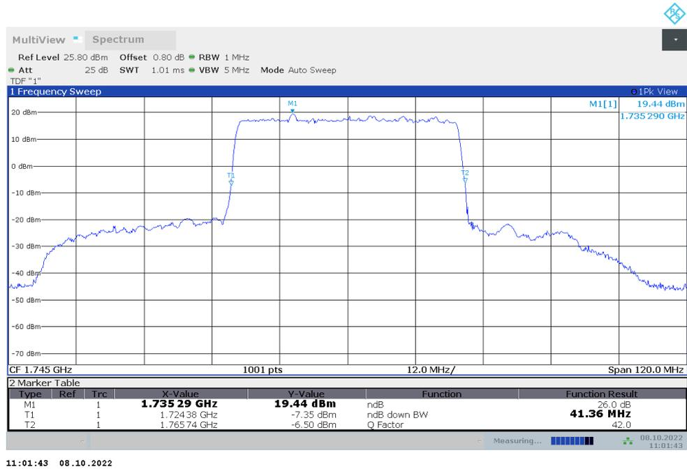
**n66,40MHz Bandwidth,DFT-s-QPSK (-26dBc BW)**
