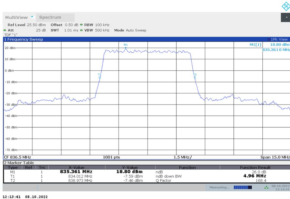
n5,5MHz Bandwidth,DFT-s-QPSK (-26dBc BW)
