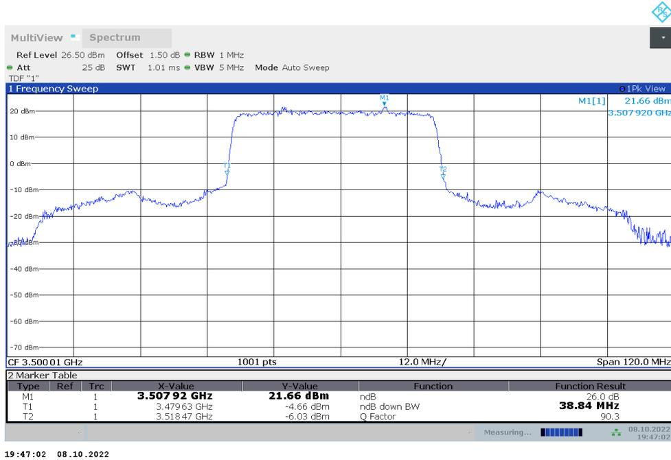
**n77L,40MHz Bandwidth,DFT-s-QPSK (-26dBc BW)**
