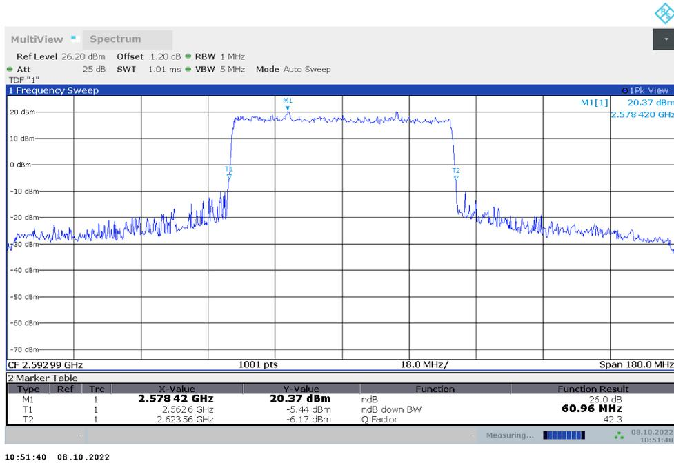
**n41,60MHz Bandwidth,DFT-s-QPSK (-26dBc BW)**
