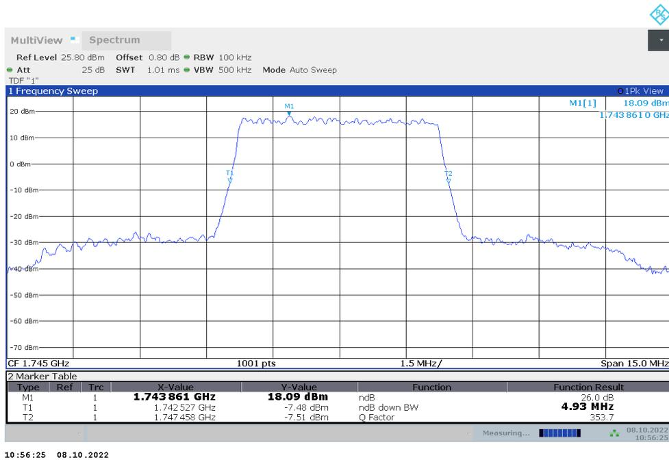
n66,5MHz Bandwidth,DFT-s-QPSK (-26dBc BW)
