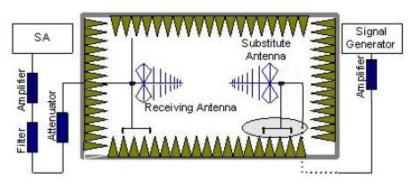
In the chamber, a substitution antenna for the frequency band of interest is placed at the reference point of the chamber. An RF Signal source for the frequency band of interest is connected to the substitution antenna with a cable that has been constructed to not interfere with the radiation pattern of the antenna. A power ( $P_{Mea}$ ) is applied to the input of the substitution antenna and adjusts the level of the signal generator output until the value of the
