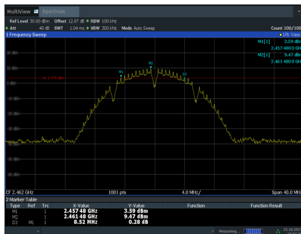
Fig.A.4.3 Occupied 6dB Bandwidth (802.11b, Ch 11)
