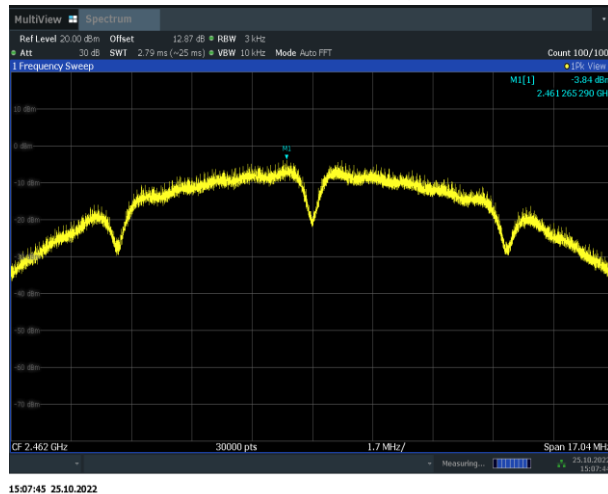
Fig.A.3.3 Power Spectral Density (802.11b, Ch 11)
