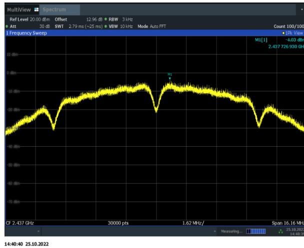
Fig.A.3.2 Power Spectral Density (802.11b, Ch 6)
