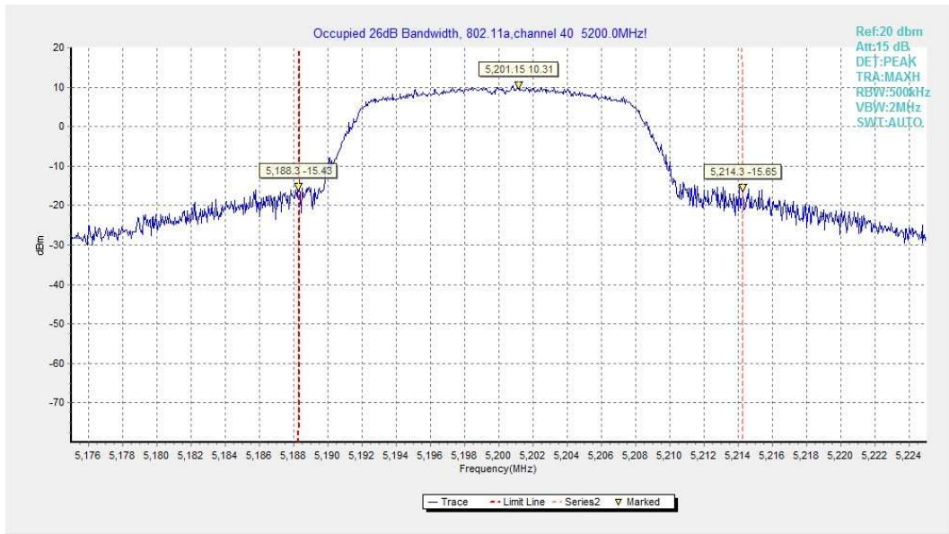
Fig.2 Occupied 26dB Bandwidth (802.11a, 5200MHz)
