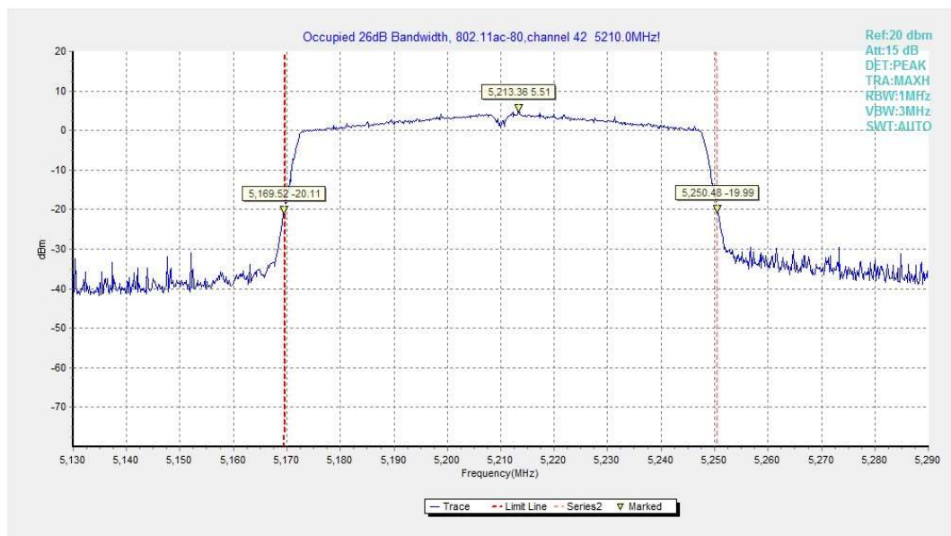
Fig.29 Occupied 26dB Bandwidth (802. 11ac-HT80, 5210MHz)
