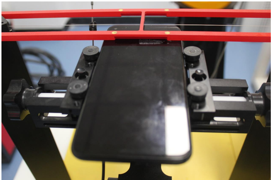
Picture 2: EUT Positioning for RF/T-coil
