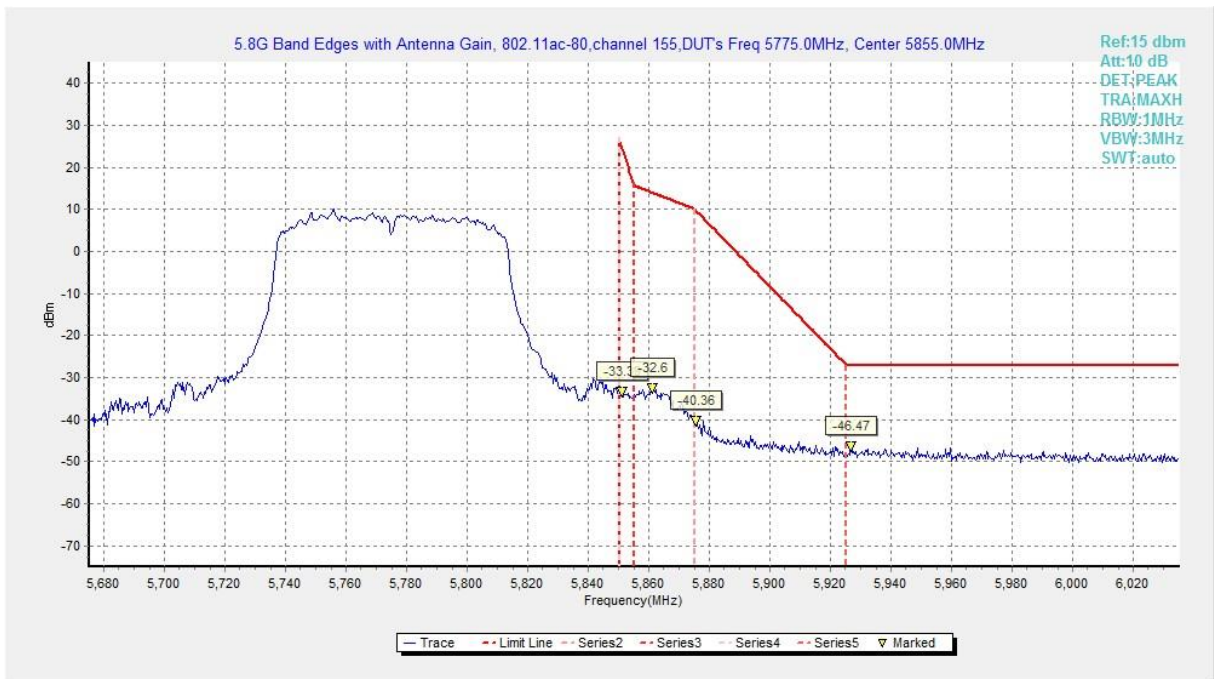
Fig. 82 Band Edges (802.11ac-HT80, 5775MHz)
