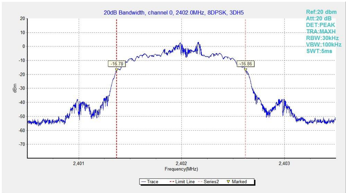
Fig.88. 20dB Bandwidth: 8DPSK, Channel 0
