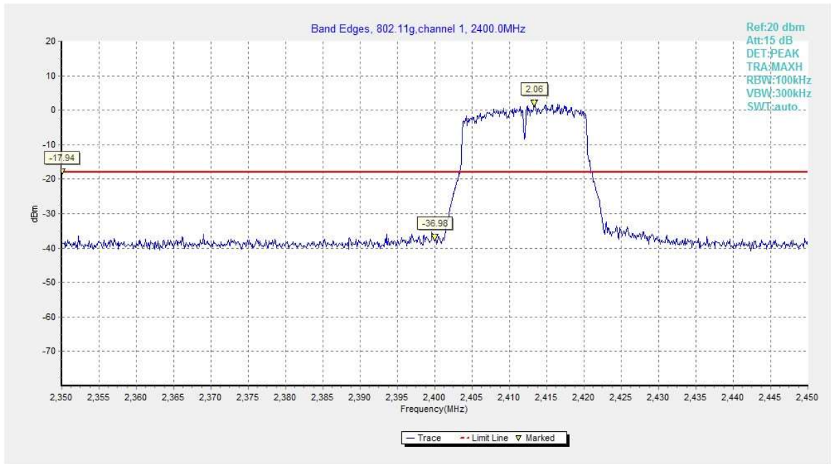
Fig.A.5.3 Band Edges (802.11g, Ch 1)
