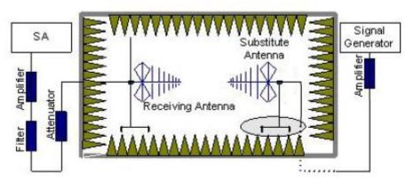
In the chamber, a substitution antenna for the frequency band of interest is placed at the reference point of the chamber. An RF Signal source for the frequency band of interest is connected to the substitution antenna with a cable that has been constructed to not interfere with the radiation pattern of the antenna. A power ( $P_{Mea}$ ) is applied to the input of the
