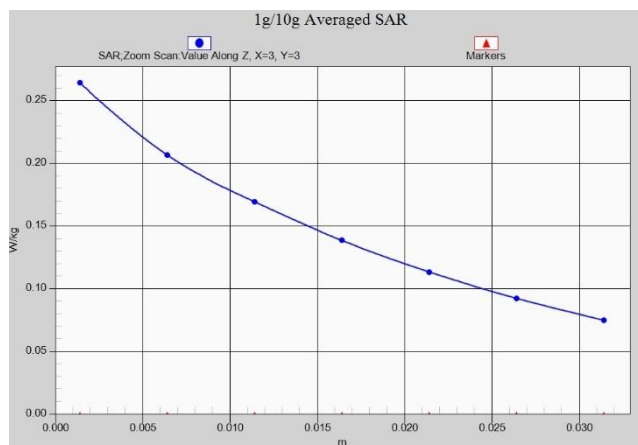
Z-Scan at power reference point (WCDMA850)
