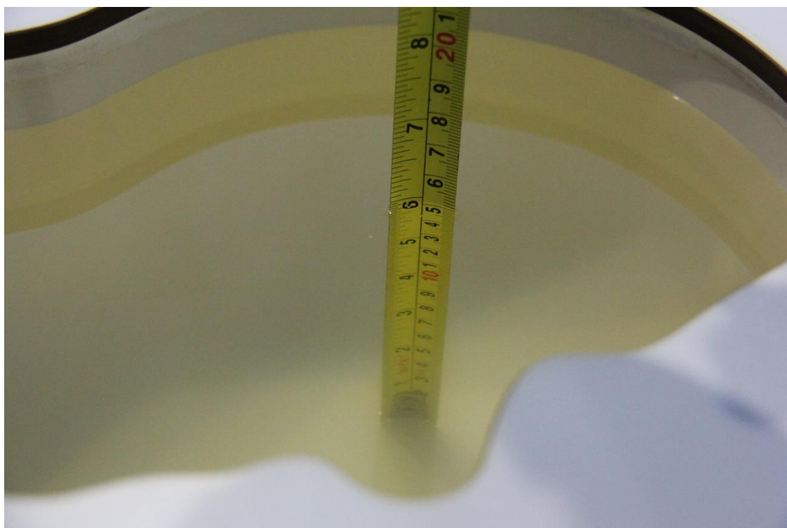
Picture 7-2 Liquid depth in the Flat Phantom (900 MHz)
