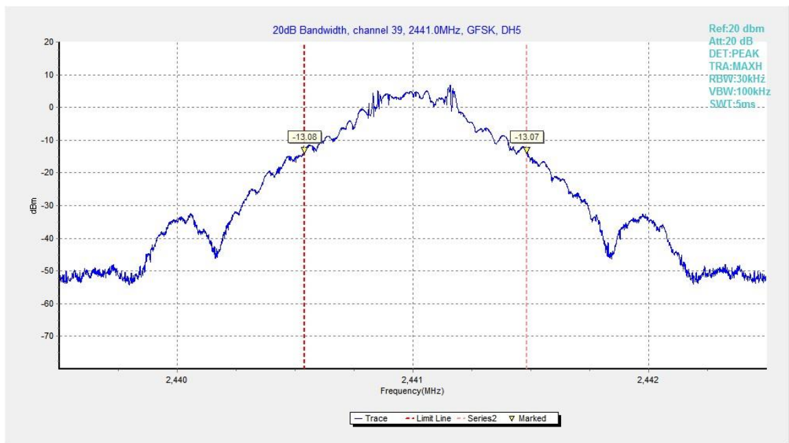
Fig.83. 20dB Bandwidth: GFSK, Channel 39
