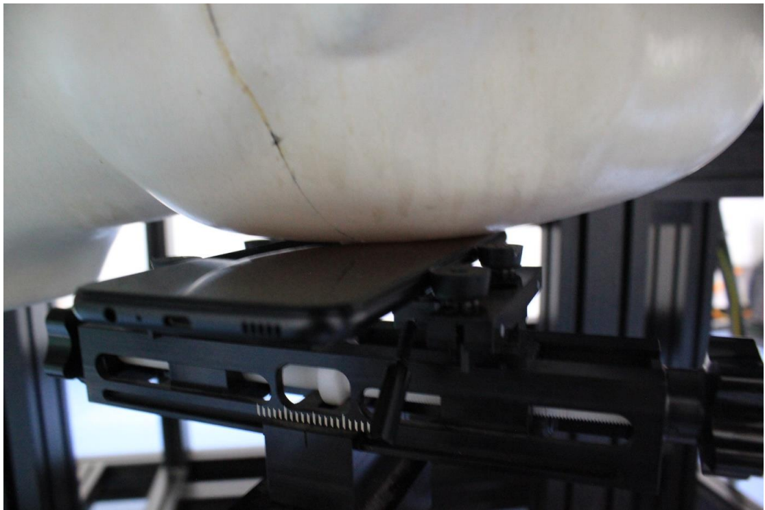
Picture 2: Left Head Touch Cheek Position
