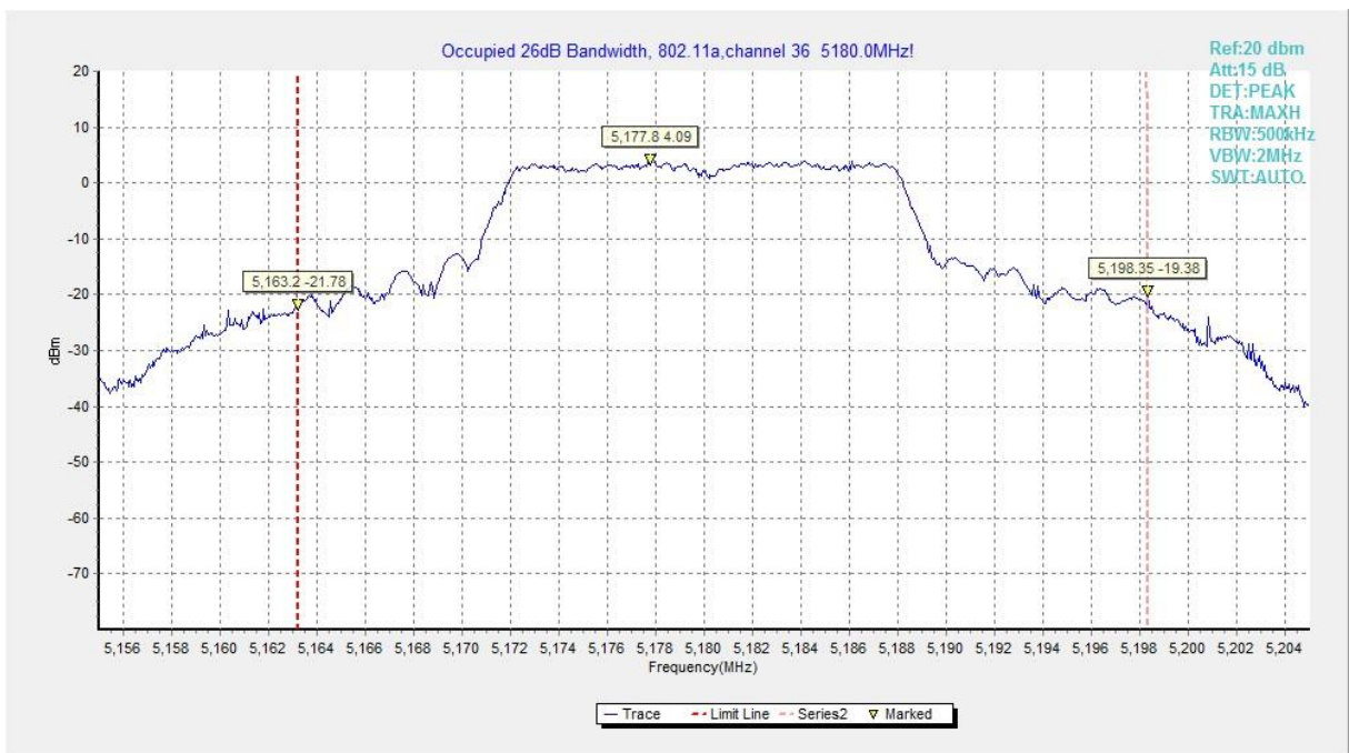
Fig.1 Occupied 26dB Bandwidth (802.11a, 5180MHz)
