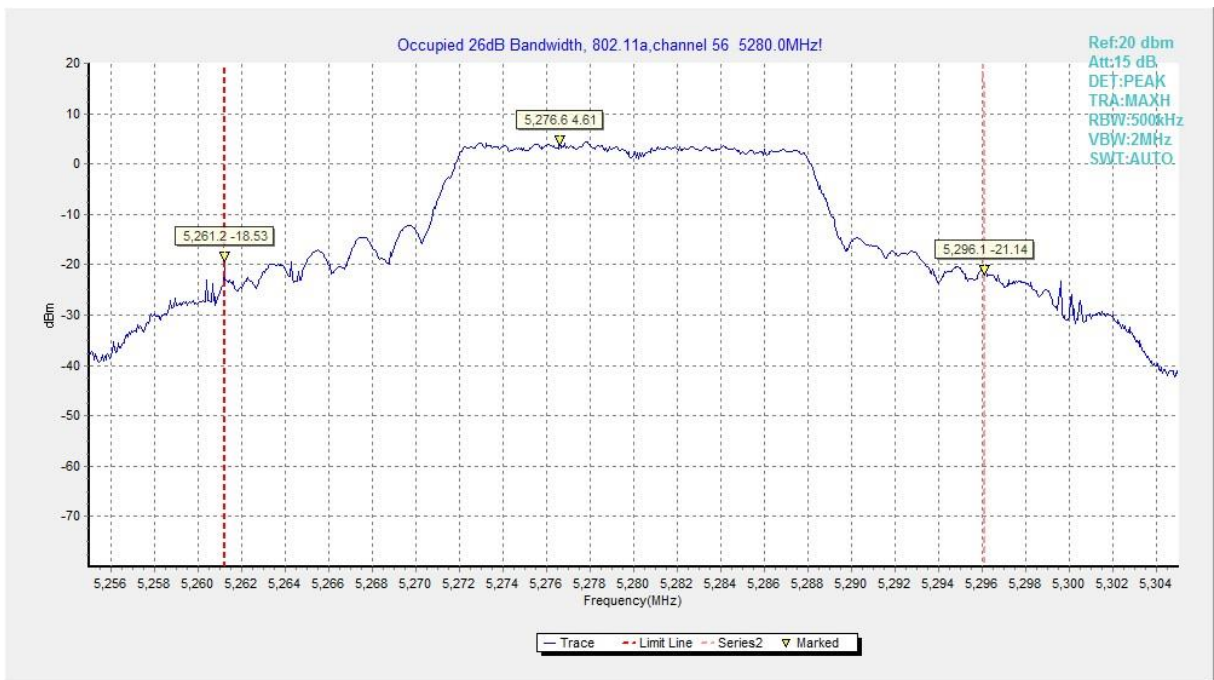
Fig.5 Occupied 26dB Bandwidth (802.11a, 5280MHz)
