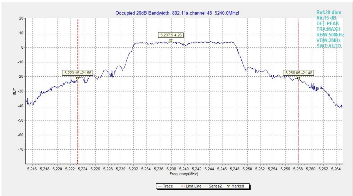
Fig.3 Occupied 26dB Bandwidth (802.11a, 5240MHz)
