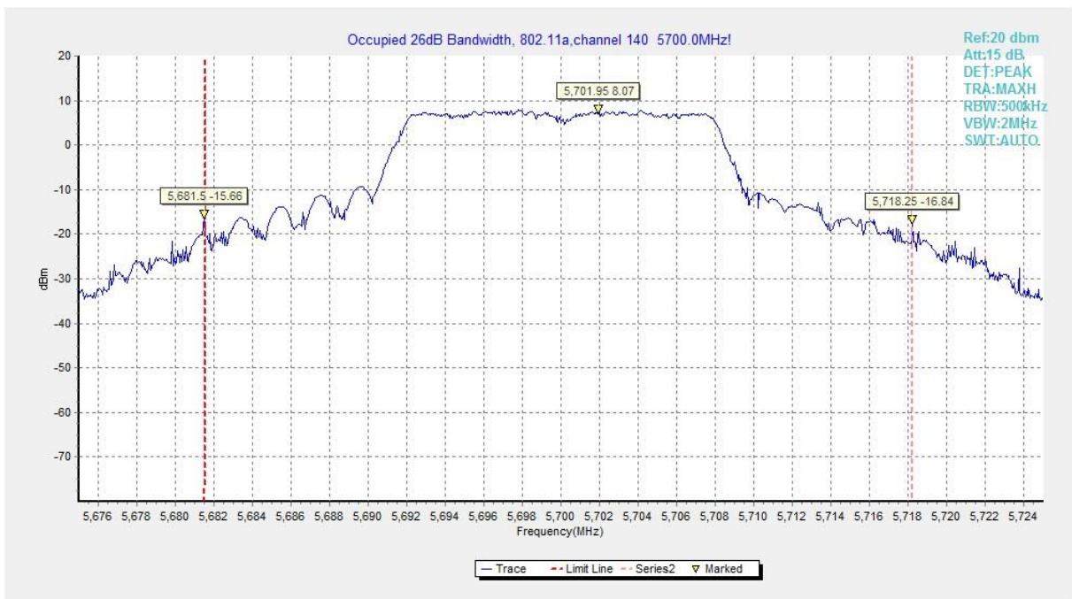
Fig.9 Occupied 26dB Bandwidth (802.11a, 5700MHz)
