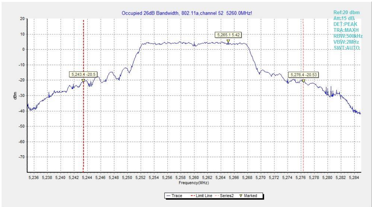
Fig.4 Occupied 26dB Bandwidth (802.11a, 5260MHz)
