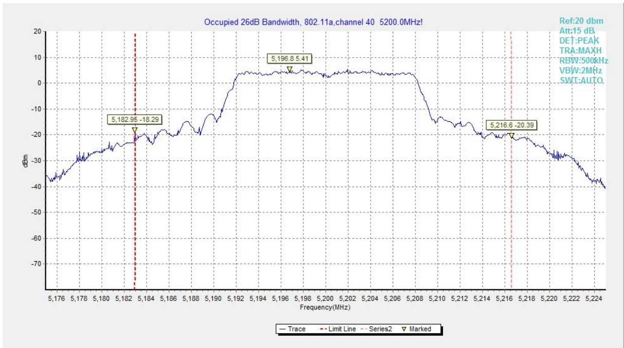
Fig.2 Occupied 26dB Bandwidth (802.11a, 5200MHz)
