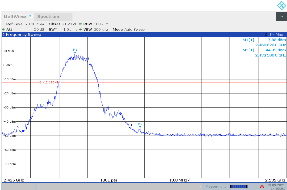
Fig.A.5.2 Band Edges (802.11b, Ch 11)
