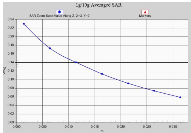
Fig.2 Z-Scan at power reference point (WCDMA850)
