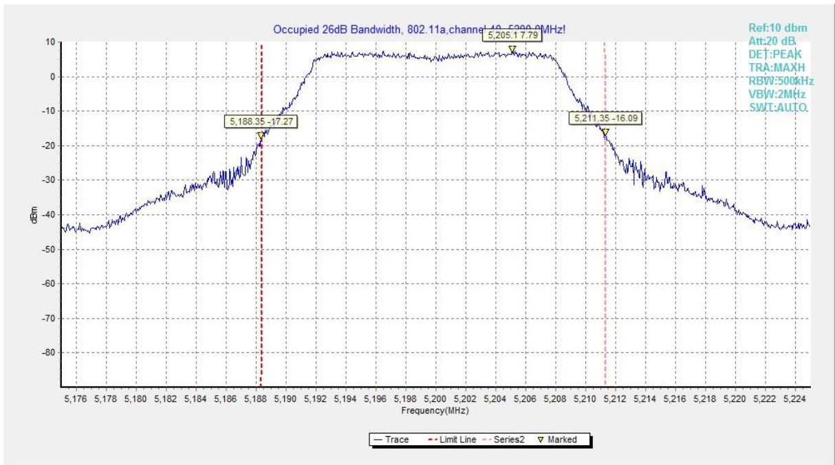
Fig.2 Occupied 26dB Bandwidth (802.11a, 5200MHz)
