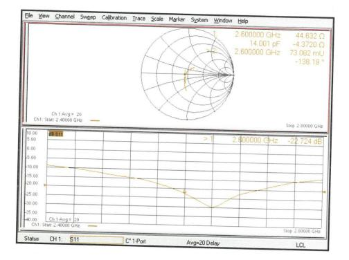
Impedance Measurement Plot for Body TSL
