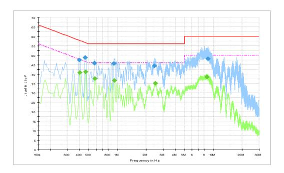
Fig.B.9.2 AC Powerline Conducted Emission-Idle
