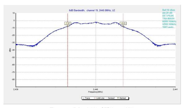
Fig.21. 6dB Bandwidth: GFSK, 2440 MHz
