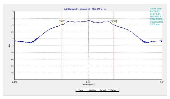
Fig.22. 6dB Bandwidth: GFSK, 2480 MHz
