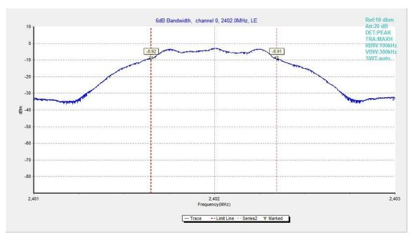
Fig.20. 6dB Bandwidth: GFSK, 2402 MHz
