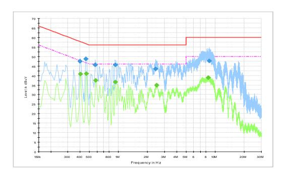
Fig.B.9.1 AC Powerline Conducted Emission- bluetooth
