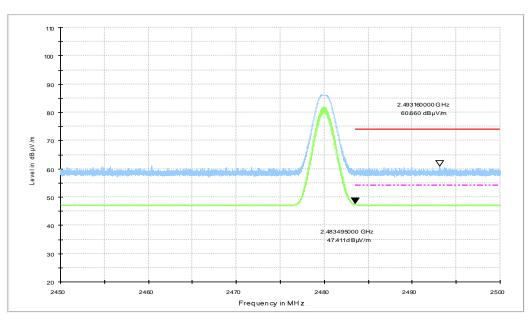
Fig.4. Frequency Band Edges: GFSK, 2480 MHz, 2.45 GHz - 2.50GHz
