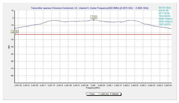
Fig.5. Transmitter Spurious Emission - Conducted: GFSK,2402MHz
