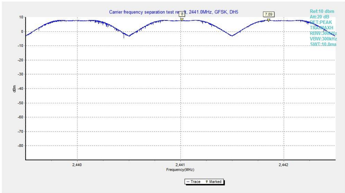
Fig.91. Carrier frequency separation measurement: GFSK, Channel 39
