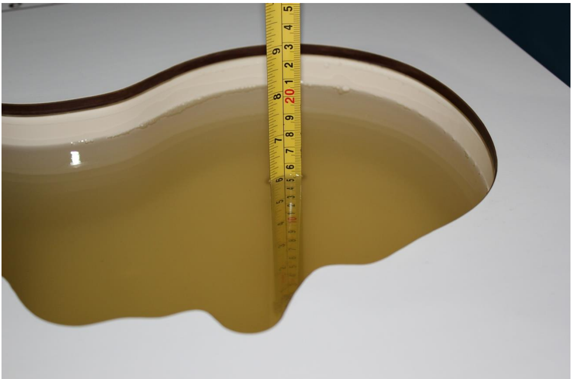
Picture 7-6 Liquid depth in the Head Phantom (2600 MHz)
