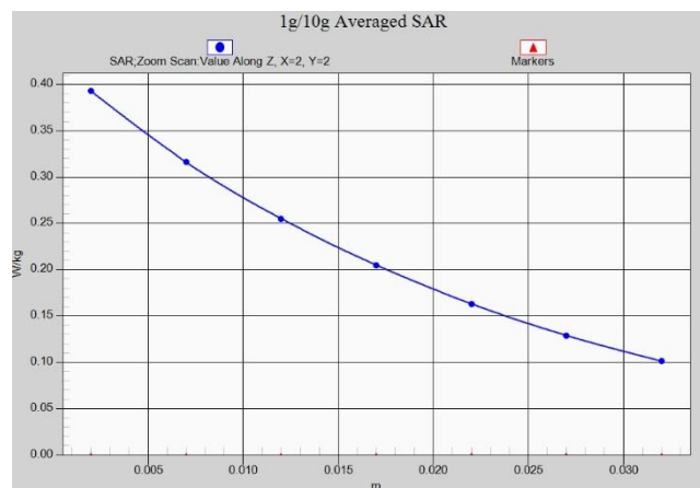
Fig. 1-9 Z-Scan at power reference point (WCDMA850 Head)
