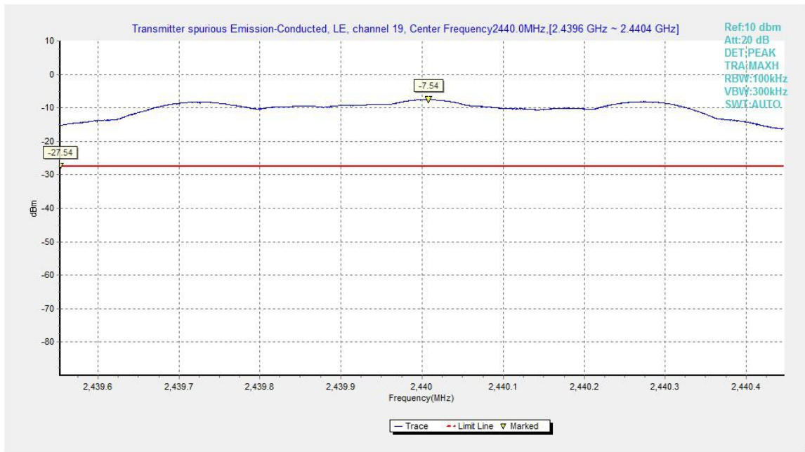
Fig.8. Transmitter Spurious Emission - Conducted: GFSK, 2440MHz
