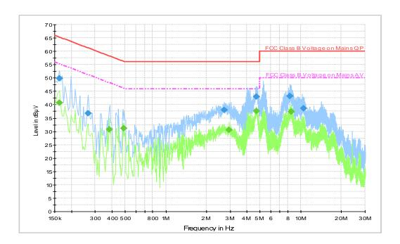
Note: The graphic result above is the maximum of the measurements for both phase line and neutral line.
