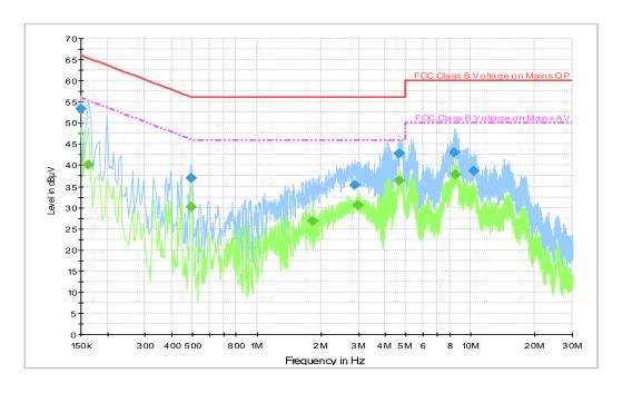
Note: The graphic result above is the maximum of the measurements for both phase line and neutral line.
