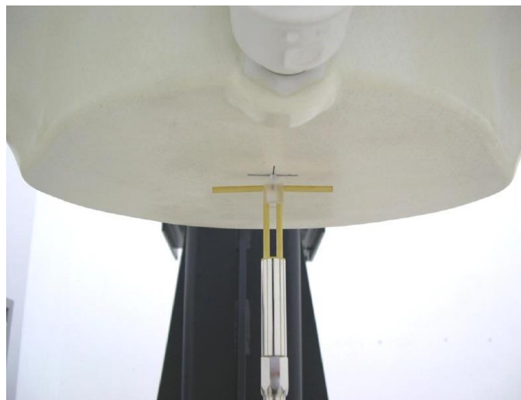
Picture 8.2 Photo of Dipole Setup
