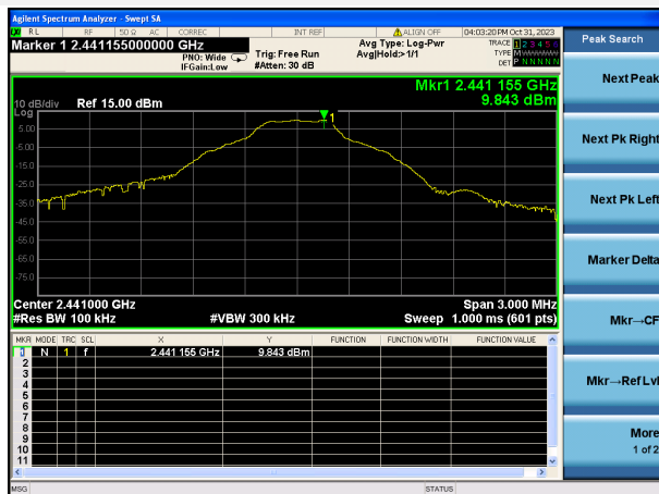
GFSK MIDDLE CHANNEL, CARRIER LEVEL
