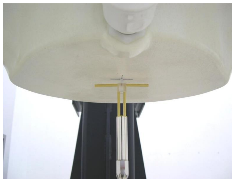
Picture 8.2 Photo of Dipole Setup
