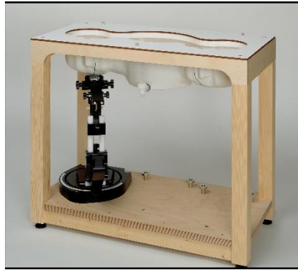
Picture C.10: SAM Twin Phantom
