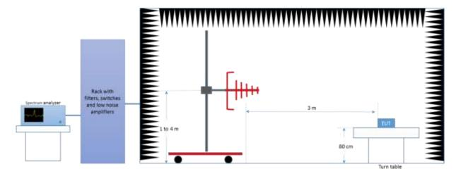
Radiated Setup 1 GHz - 6.4 GHz
