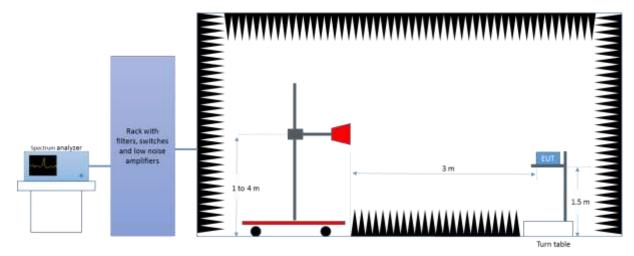
Radiated Setup 6.4 GHz - 18 GHz
