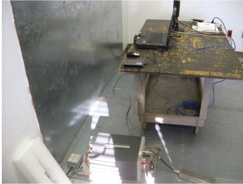
Test Setup – Conducted Emissions - MAINS
