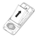
Warning: Make sure to power off the phone before taking out SIM card, battery, otherwise your SIM card might be damaged.
