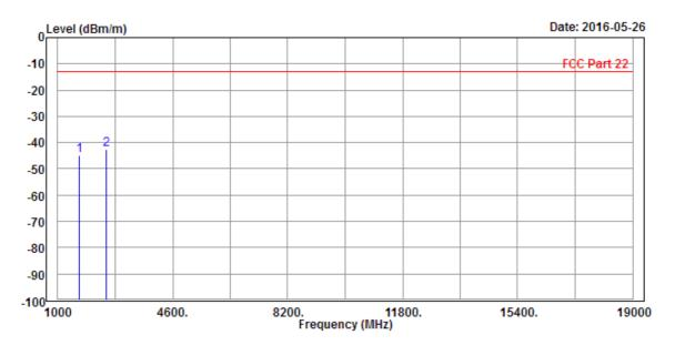
Condition: FCC Part 22 3m EIRP\_1G-18G-\_20160505-EMC012645B+3117-FCC Horizontal
