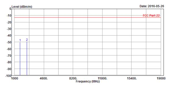
Condition: FCC Part 22 3m EIRP\_1G-18G-\_20160505-EMC012645B+3117-FCC Horizontal
