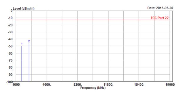
Condition: FCC Part 22 3m EIRP\_1G-18G-\_20160505-EMC012645B+3117-FCC Vertical
