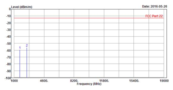
Condition: FCC Part 22 3m EIRP\_1G-18G-\_20160505-EMC012645B+3117-FCC Horizontal
