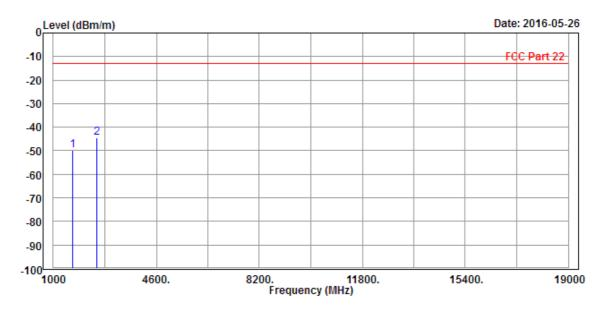
Condition: FCC Part 22 3m EIRP\_1G-18G-\_20160505-EMC012645B+3117-FCC Vertical
