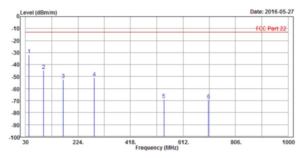
Condition: FCC Part 22 3m EIRP\_26M-1GHz-20160505-EMC9135+3143B-FCC Horizontal
