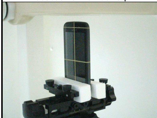
Top Side of EUT with 1.0 cm Gap
